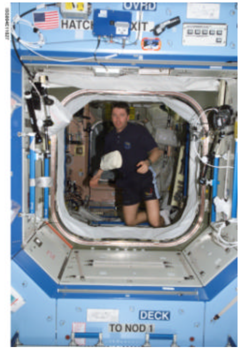
Endcone with closeouts in place
