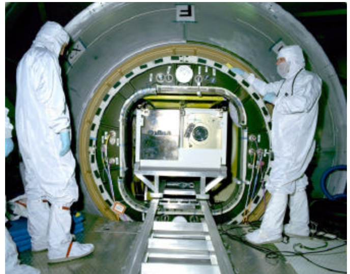
Rack being installed in the module
