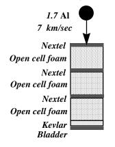
Figure 8. TransHab Orbital Debris Shield
