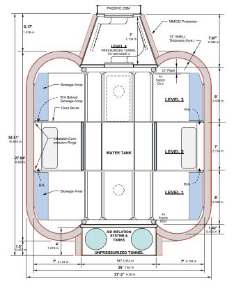
Figure 1. ISS TransHab Section
