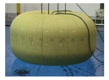
Figure 9. TransHab Hydrostatic Test
