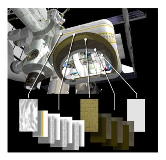
Figure 7. TransHab Demonstrates Large Diameter Inflatable Structure
