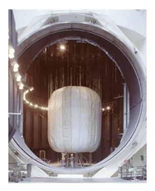
Figure 10: TransHab Vacuum Deployment Test
