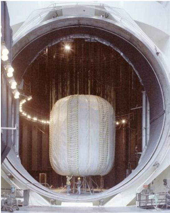
Figure 10: TransHab Vacuum Deployment Test
