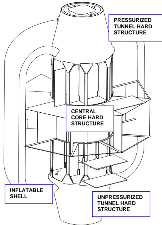
Figure 6. TransHab Assembled Core within the Inflated Shell
