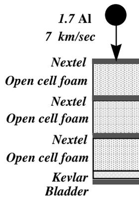
Figure 8. TransHab Orbital Debris Shield
