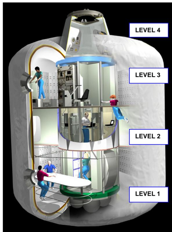
Figure 2. ISS TransHab Internal View
