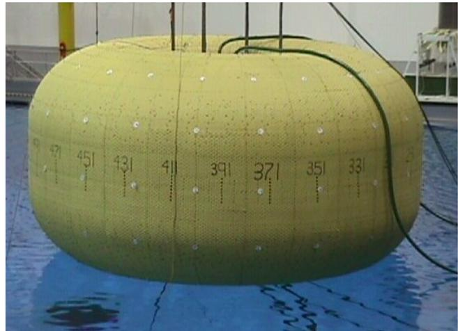
Figure 9. TransHab Hydrostatic Test
