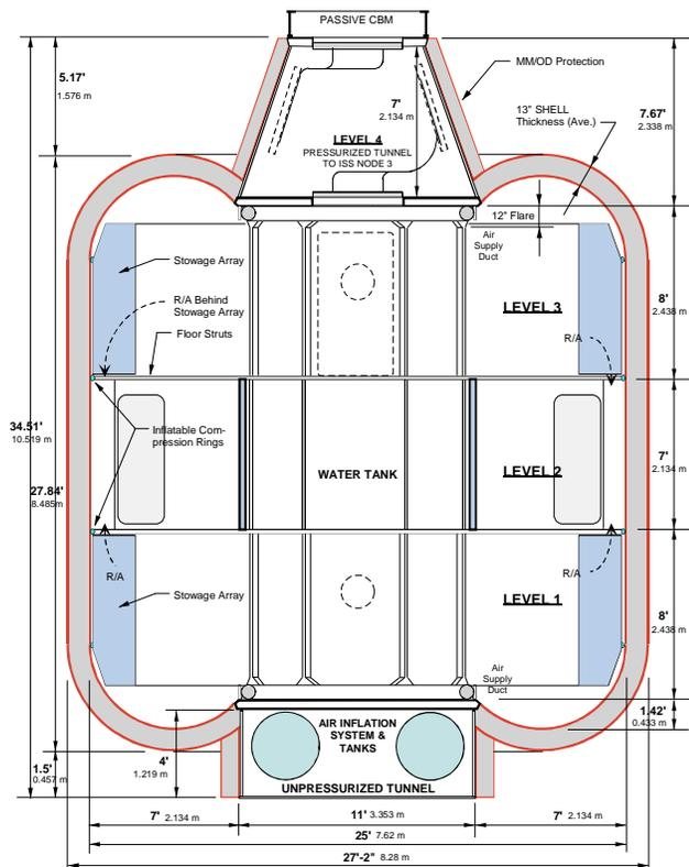
Figure 1. ISS TransHab Section
