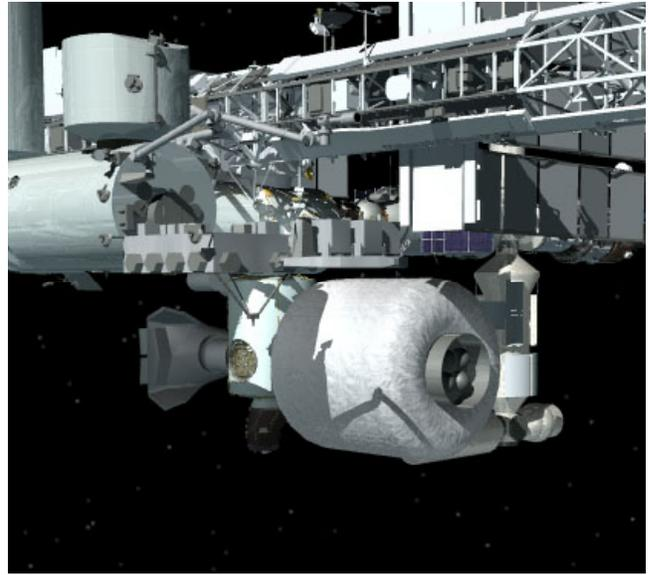
Figure 11. Proposed ISS TransHab on Space Station
