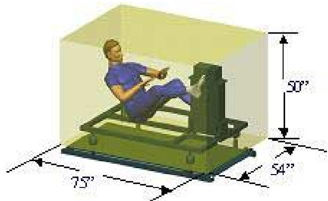
FIGURE 4: The Cycle-Ergometer with Vibration Isolation System (CEVIS) mounts to the front face of a rack. It is as wide as a rack, has a significant operational envelope (as shown), and has a dynamic range-of-motion that overlaps onto adjoining rack faces by 6.25" in each lateral direction. CEVIS is the largest rack-based protrusion that IVC has yet had to integrate.
