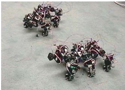
Figure 1a: CONRO modules in spider configuration. http://www.isi.edu/conro
