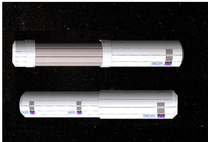
**Figure 2. Expandable Modules in Deployed Configuration.**
