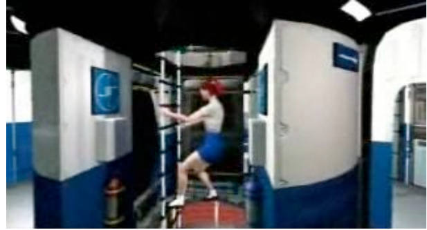
Figure 27. Scenes from a computer animation of a TransHab module in an artificial-gravity crew transfer vehicle. From the “Bimodal NTR Artificial Gravity Mars Mission” produced by NASA Glenn Research Center and John Frassanito & Associates [Borowski, Dudzinski, Sauls, Minsaas, 2006]. With 0.38 g at 4 rpm, the top floor radius would be 21.2 m with a tangential velocity of 8.9 m/s. Under these conditions, the apparent floor slope when walking west at 1 m/s would be as much as 13° (23% grade, 1:4.33). The apparent lean of the ladder when descending at 0.5 m/s would be more than 6° from vertical. Due to the reversal of Coriolis acceleration in ascending versus descending, one ladder cannot provide safe transit in both directions.
