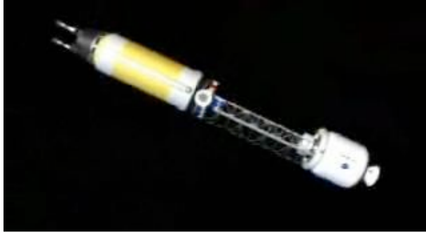
Figure 27. Scenes from a computer animation of a TransHab module in an artificial-gravity crew transfer vehicle. From the “Bimodal NTR Artificial Gravity Mars Mission” produced by NASA Glenn Research Center and John Frassanito & Associates [Borowski, Dudzinski, Sauls, Minsaas, 2006]. With 0.38 g at 4 rpm, the top floor radius would be 21.2 m with a tangential velocity of 8.9 m/s. Under these conditions, the apparent floor slope when walking west at 1 m/s would be as much as 13° (23% grade, 1:4.33). The apparent lean of the ladder when descending at 0.5 m/s would be more than 6° from vertical. Due to the reversal of Coriolis acceleration in ascending versus descending, one ladder cannot provide safe transit in both directions.
