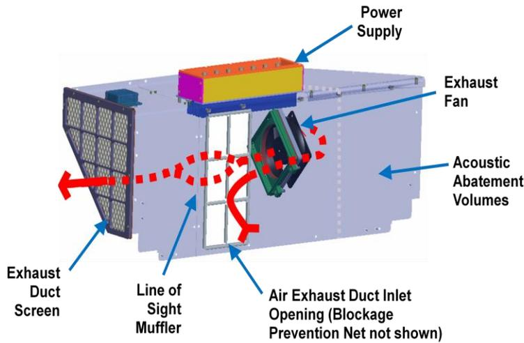
**Figure 5. Exhaust duct ventilation flow path and volume dedicated to abatements.**
