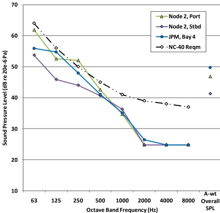
Figure 19. On-orbit CQ interior sound-level measurements at the crew member head location with the fan on low fan speed.
