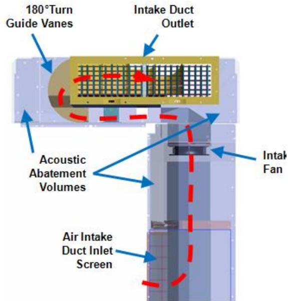
**Figure 4. Intake duct ventilation flow path and volume dedicated to abatements.**
