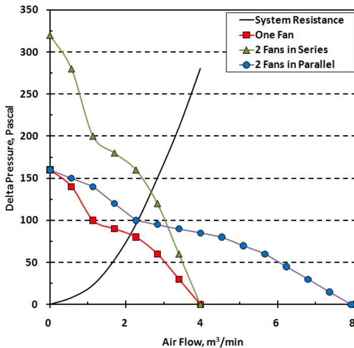
**Figure 6. CQ fan performance for single, serial, and parallel configurations.**
