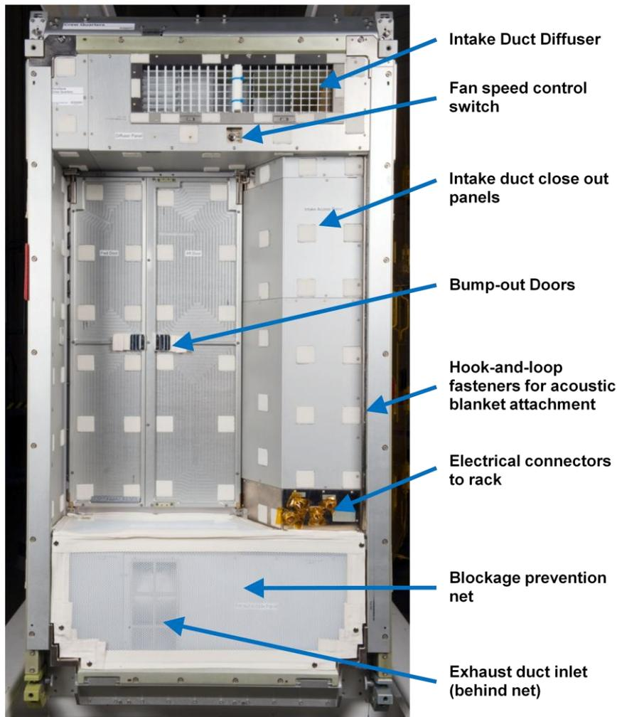
**Figure 2. Deck CQ in the launch configuration.**
