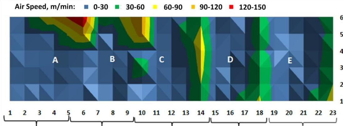
**Figure 11. Airspeed at each opening in air diffuser outlet after addition of flow vanes to create five air channels (A through E).**
