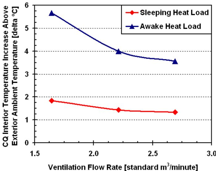
Figure 8. Temperature rise verses flow rate.<sup>2</sup>
