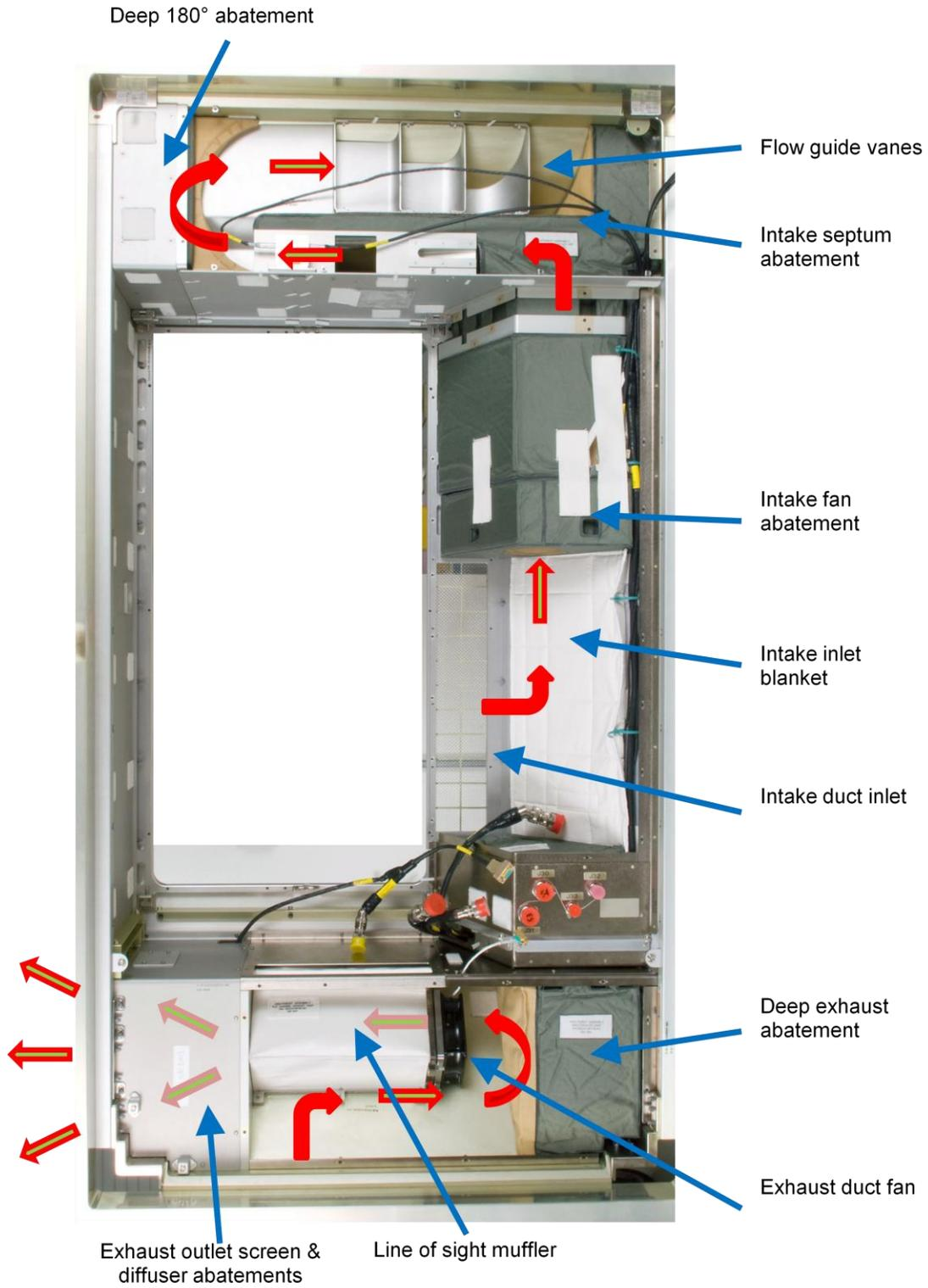
**Figure 15. Bump-out interior with acoustic blankets and closeout panels removed to expose ventilation duct acoustic abatements.**
