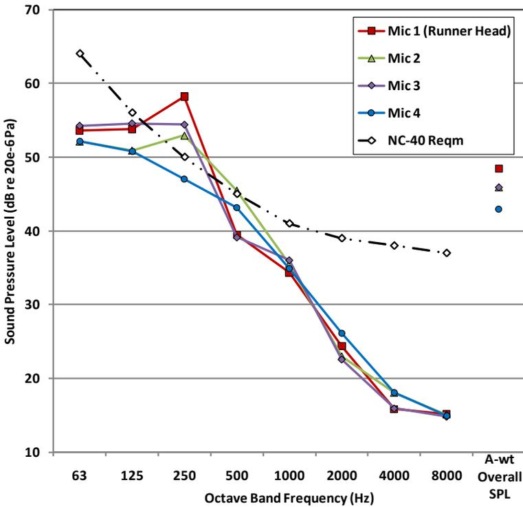
Figure 18. CQ interior sound-level measurements at low fan speed from microphone array.
