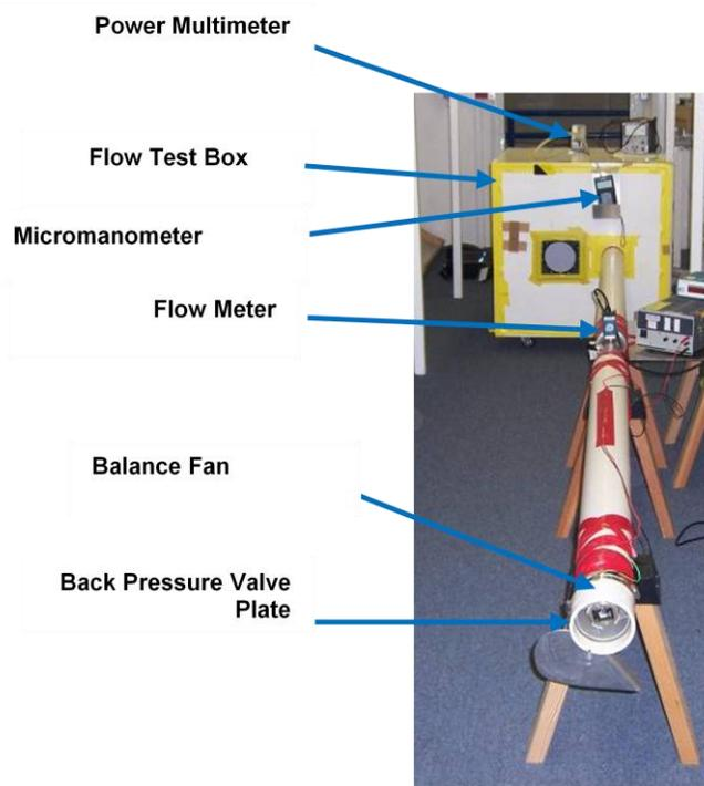
Figure 7. CQ fan flow performance test stand.
