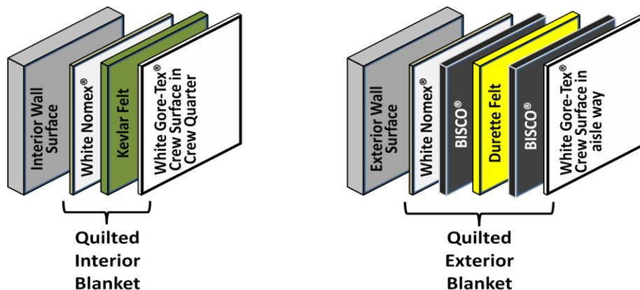
**Figure 13. Interior (left) and exterior (right) acoustic blanket material layers.**
