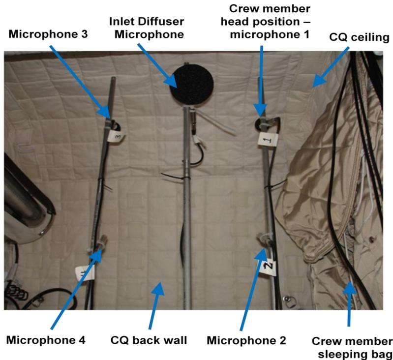
Figure 17. Photograph of the CQ interior 30 cm measurement grid.
