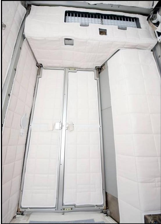
**Figure 3. Port/Deck CQ interior in the on-orbit deployed configuration.**
