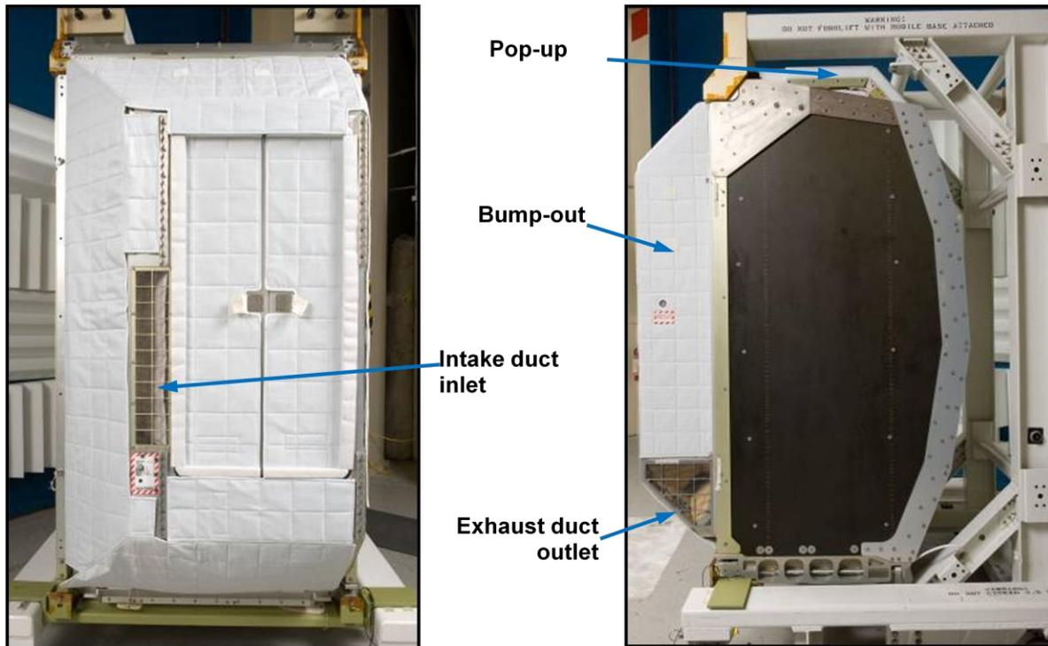
**Figure 1.** External view of front side toward aisleway (left) and aft side (right) of Deck CQ on-orbit configuration in a rack handling adapter (white structure).
