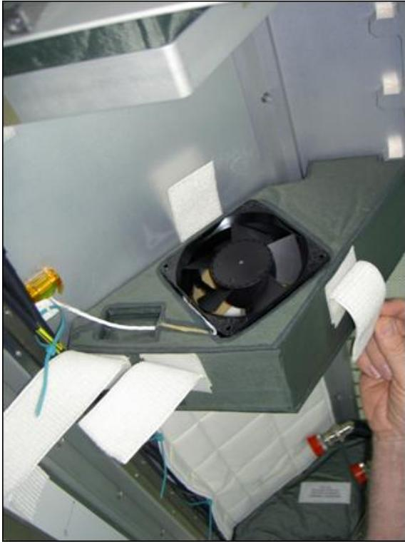
**Figure 12. Intake fan soft captured in foam abatement.**
