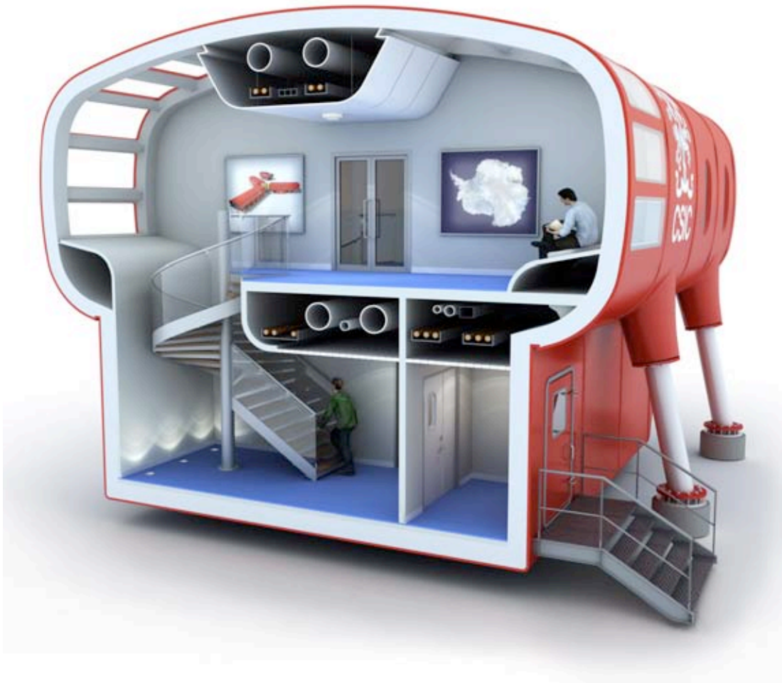
Figure 13. Cross sectional visualization taken through entry stairs showing service distribution at ground level between floors, service distribution across glazed stair foyers at first floor level, FRP legs supported on precast concrete foundations and lobbied entrances
