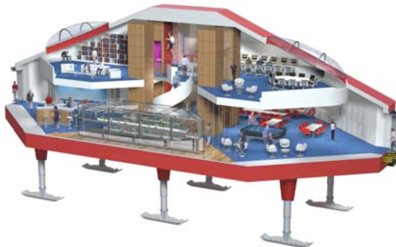
Figure 2. Cut away visual of the central module, which provides space for recreation and relaxation. In the final design the gymnasium is placed on the upper level and the climbing wall was omitted for health and safety reasons (as it is also next to the bar!)
