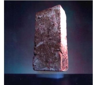
Figure 3. Aerogel supporting a brick. Courtesy NASA/JPL-Caltech
