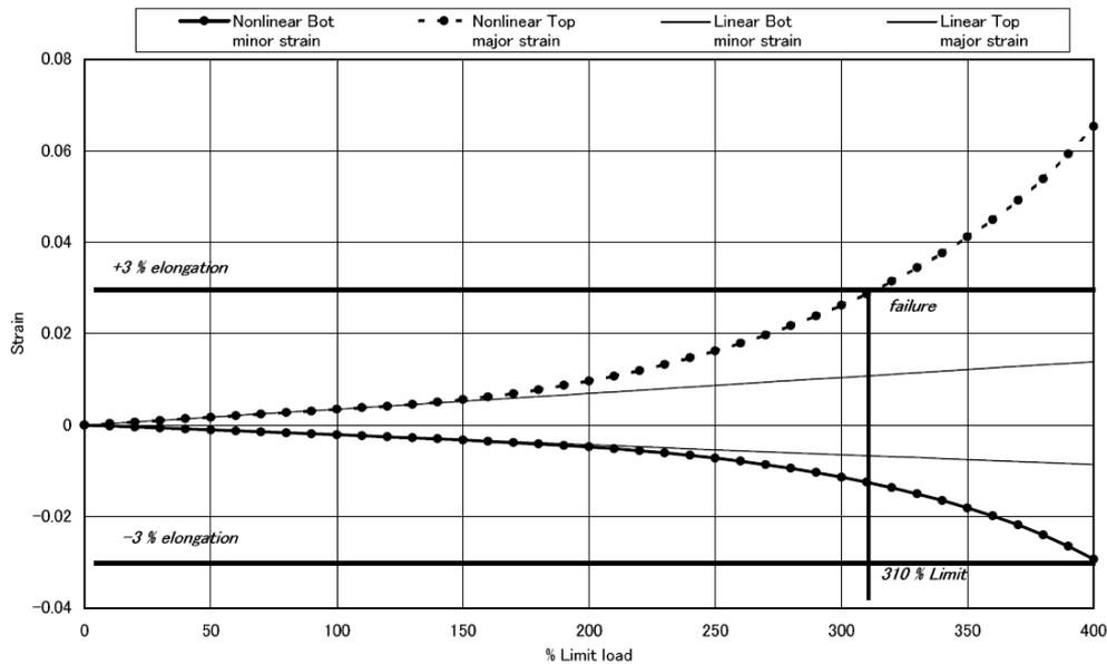
**Figure 6. Result of non-linear analysis for keel trunnion**
