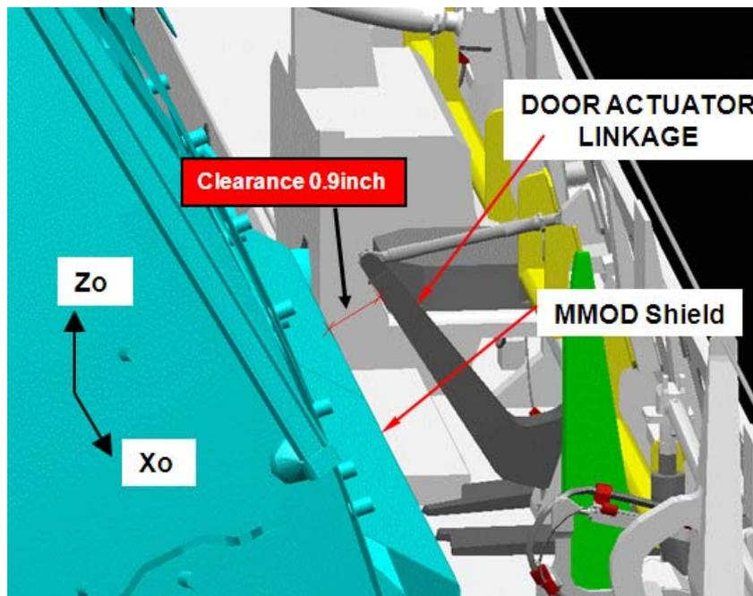
**Figure 2. A sample of Dynamic Clearance of PM and Space Shuttle**
