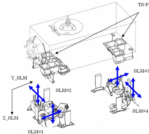
**Figure 14. SLM configuration for supporting trunnion**
