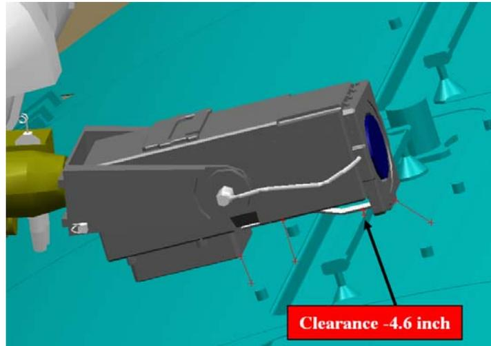
**Figure 7. Interference of SRMS elbow camera to handrail**
