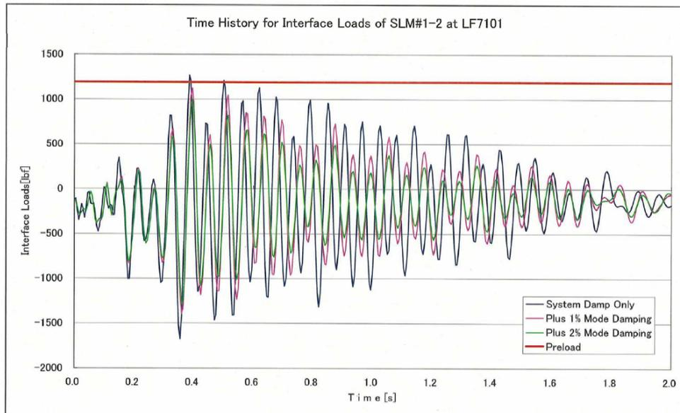
**Figure 16. Comparison between preload and response**
