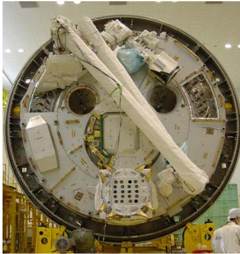
**Figure 9. Main Arm installed to PM (Flight Configuration)**
