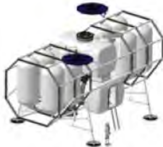
FIGURE 7. Alternate Lunar Lander Configuration. This arrangement of Ascent Module and “wing tanks” above the Habitat can increase radiation shielding on the surface, drawing credit: Rush Wofford.
