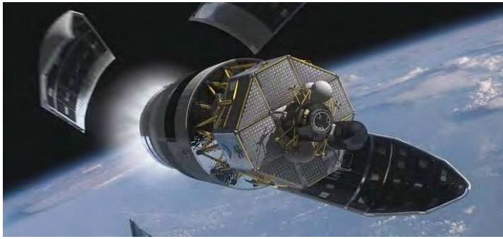
NASA Altair Lunar Lander: Shroud Separation before Trans-Lunar Injection
