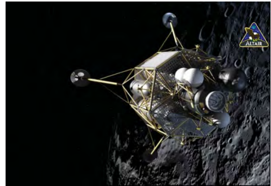
NASA Altair Lunar Lander after separation from the Orion CEV during terminal descent and landing.
