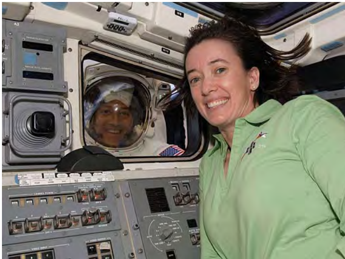
FIGURE 14 suggests another aspect of windows for crew operations. The figure shows a photo of two shuttle astronauts, one IVA at the Aft Flight Deck that looks out on the cargo bay and the other from which the crewmembers operate the robotic arm. Looking in through the aft window is an EVA astronaut. FIGURE 14 provides both an example and a counter-example, the example being of a crewmember potentially using the window to monitor the EVA activities of fellow crew.
