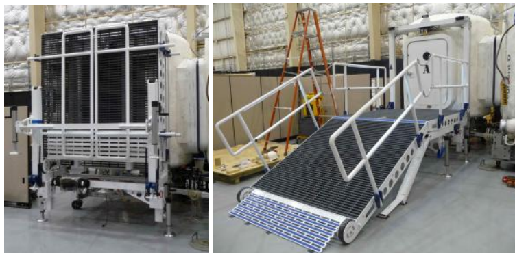
Figure 13. EVA Porch Integrated with Airlock (right deployed, left stowed)
