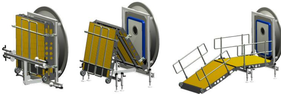
Figure 9. EVA Porch deployment (1 st concept)
