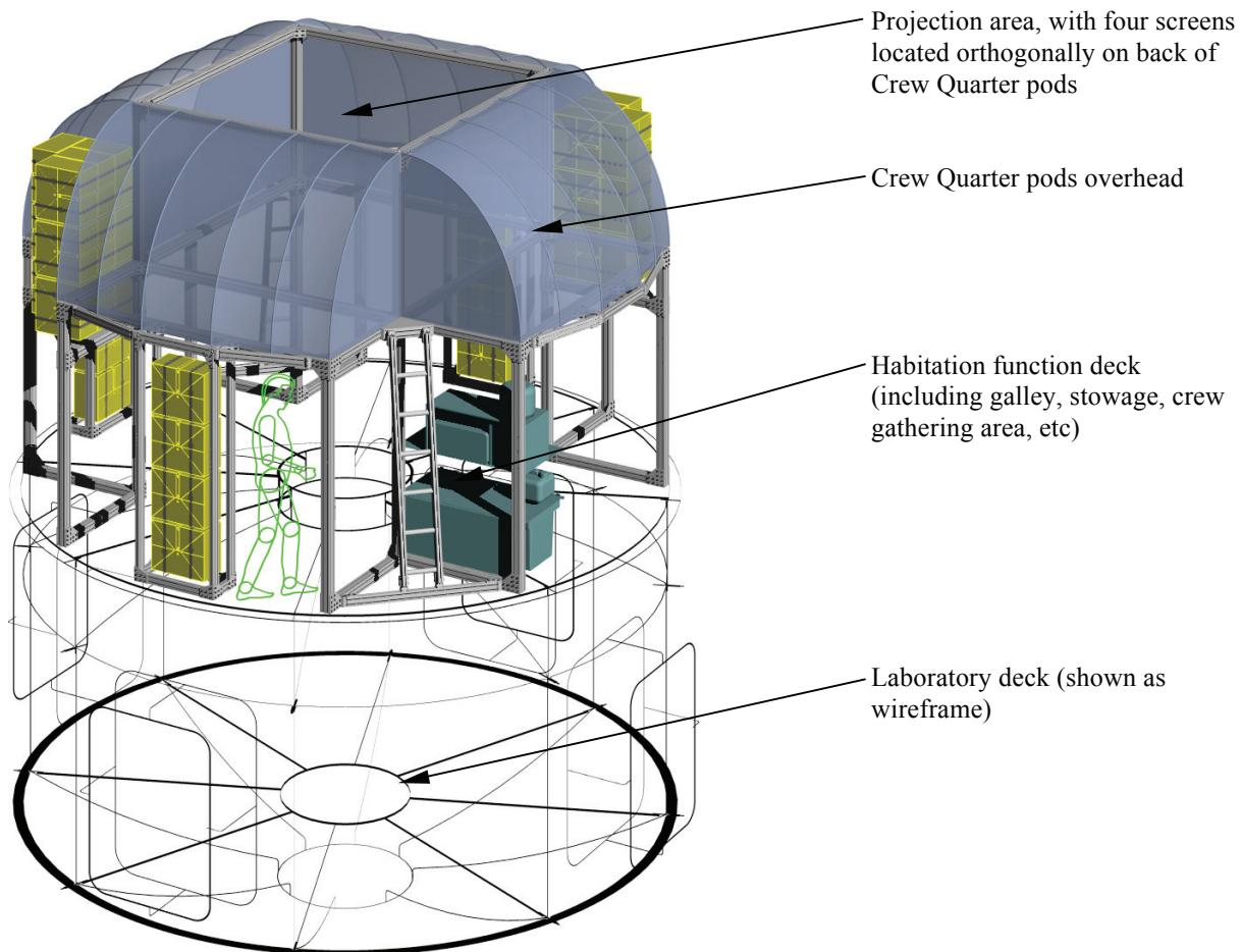
**Figure 2: HDU-DSH X-Hab Loft configuration**
