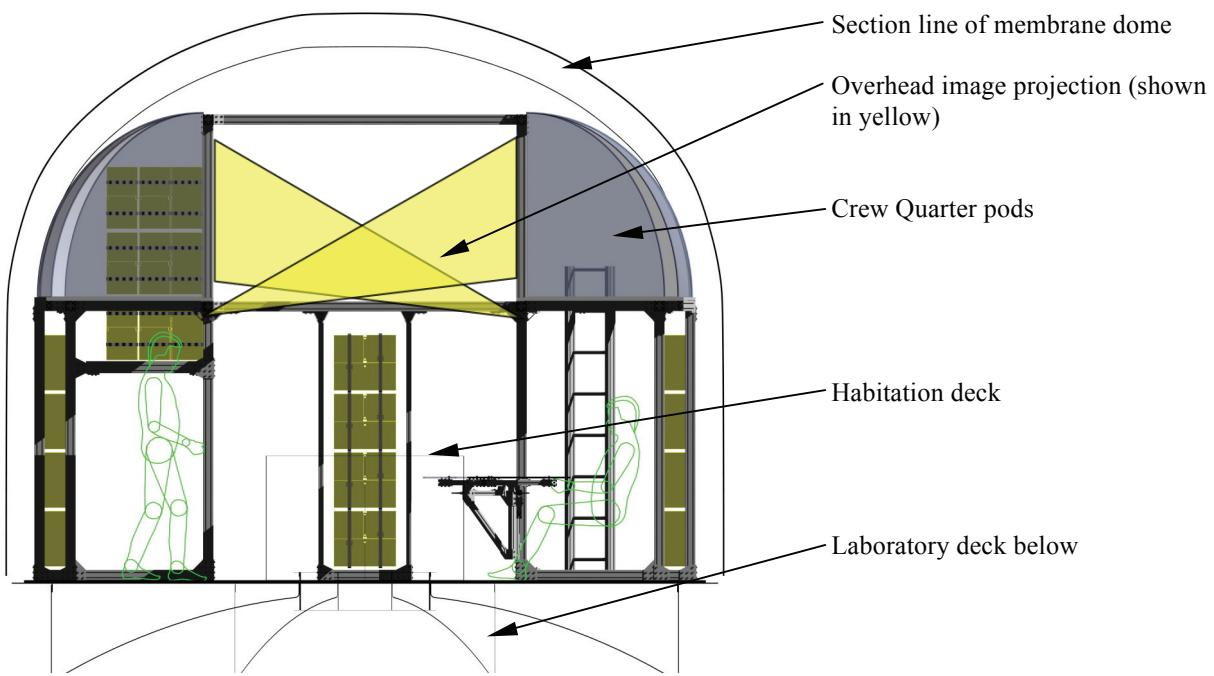
**Figure 3: HDU-DSH projector screen CAD configuration**
