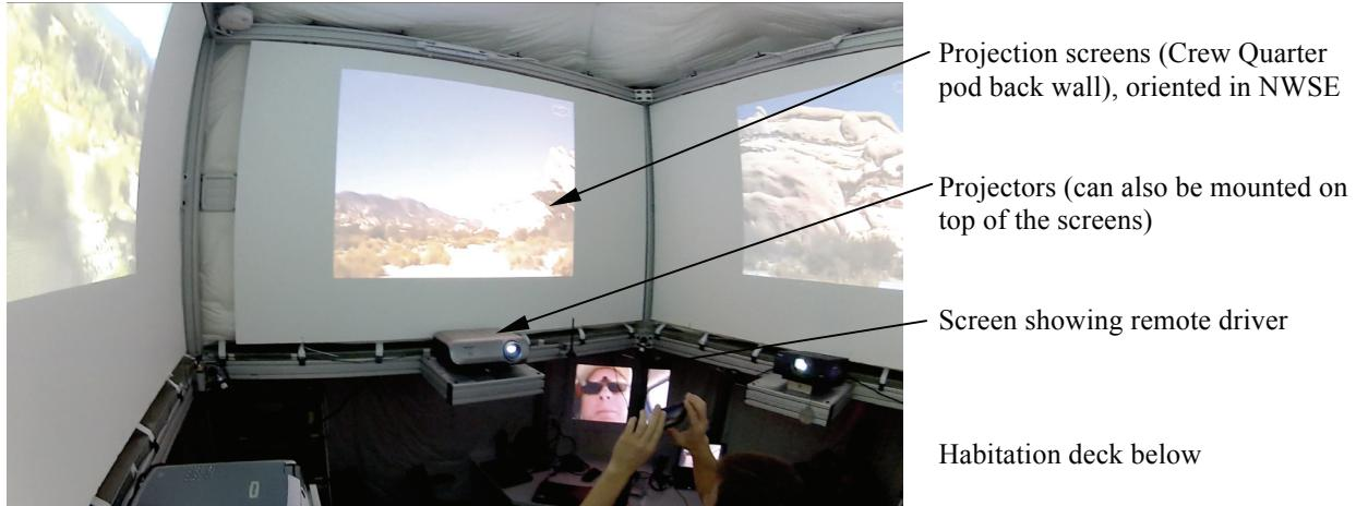
**Figure 4: HDU-DSH projector screen in use**
