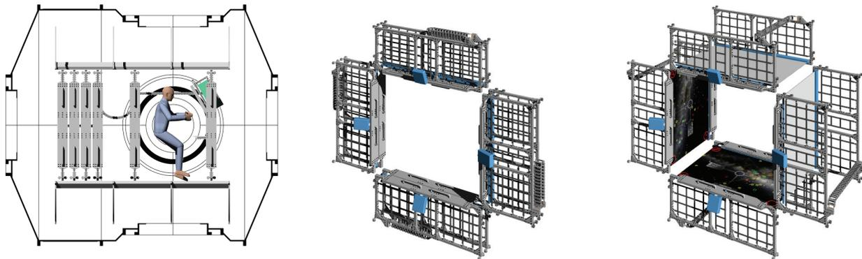
Figure 12: Random Access Frame (RAF) layout inside an ISS-based Node 1 module (left), with Virtual Window stowed (middle), and deployed (right)
