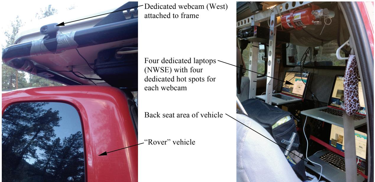
**Figure 7: Simulated rover setup, exterior (left) and interior (right)**
