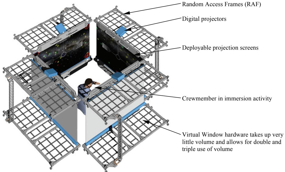
**Figure 13: Lightweight projection screens used as a Virtual Window showing crew in immersion activity**
