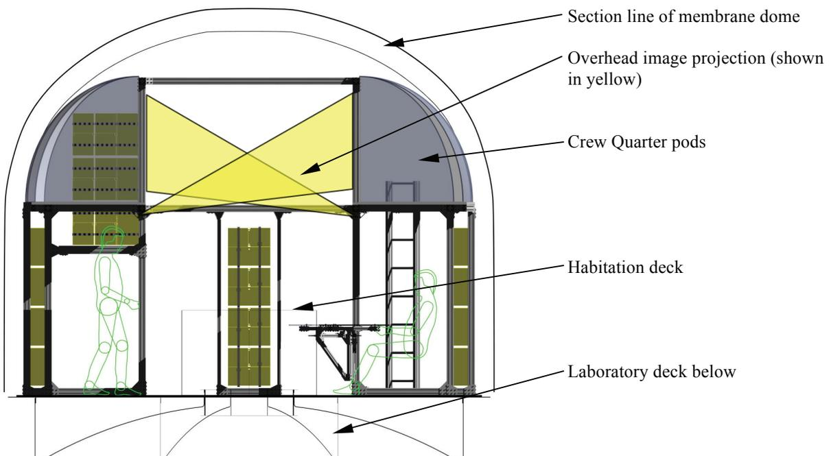
**Figure 3: HDU-DSH projector screen CAD configuration**
