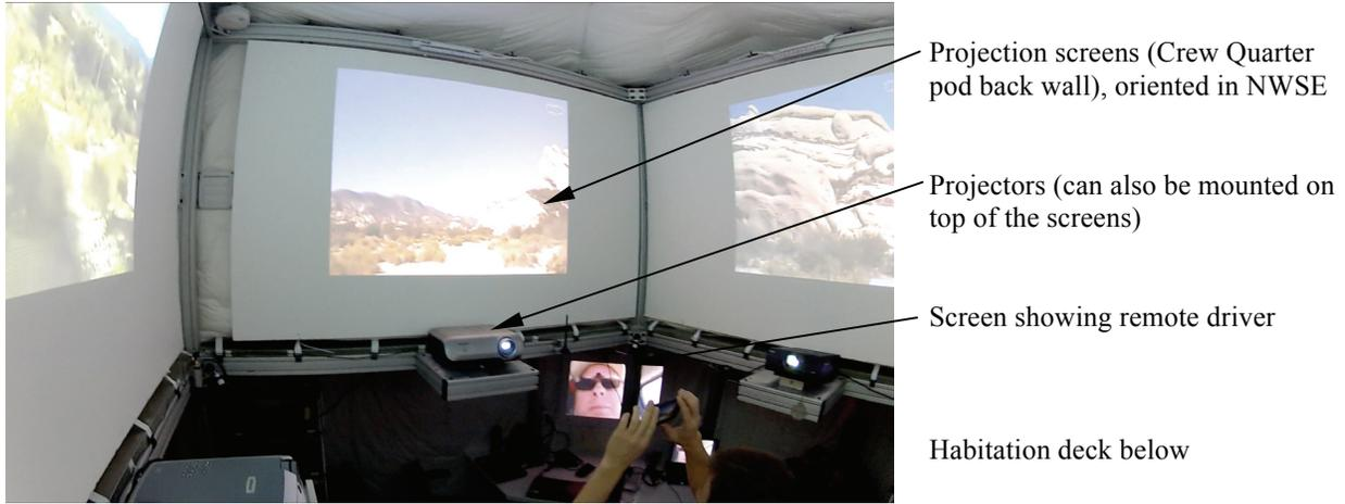
**Figure 4: HDU-DSH projector screen in use**
