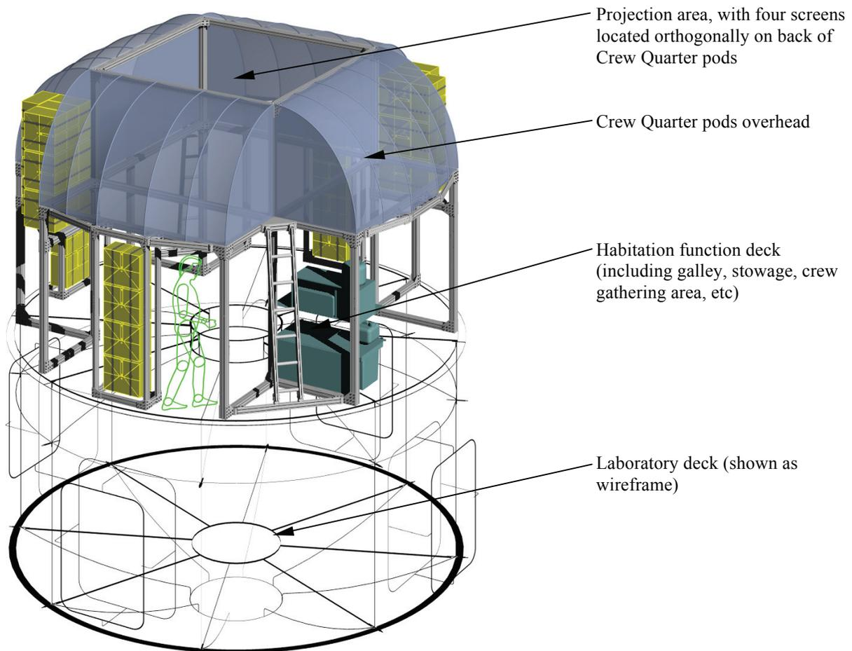
**Figure 2: HDU-DSH X-Hab Loft configuration**
