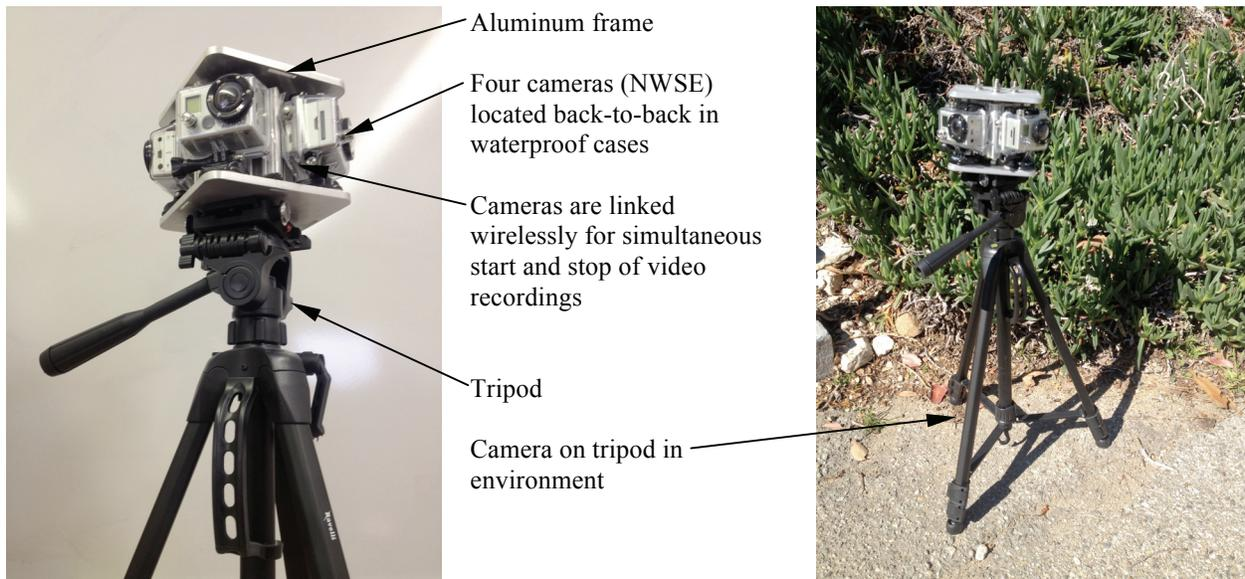
**Figure 10: Camera for preparing pre-recorded nature scenes projected into HDU-DSH**
