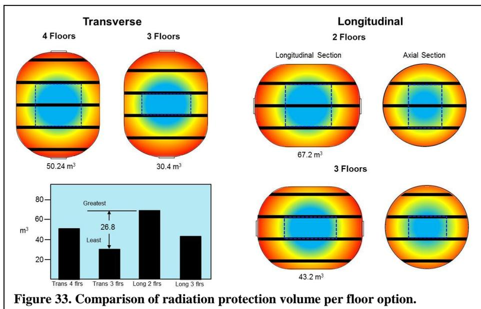
**Figure 33. Comparison of radiation protection volume per floor option.**
