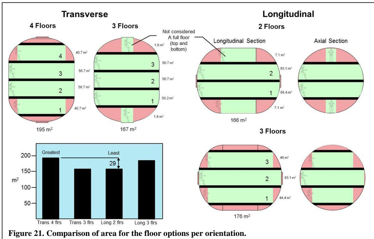
**Figure 21. Comparison of area for the floor options per orientation.**
