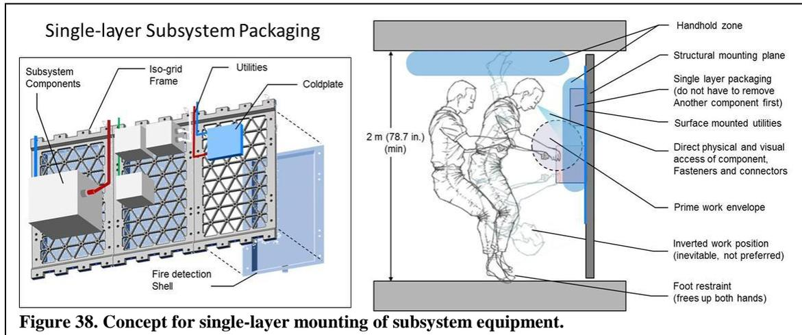
**Figure 38. Concept for single-layer mounting of subsystem equipment.**
