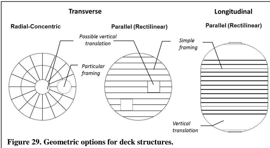
**Figure 29. Geometric options for deck structures.**
