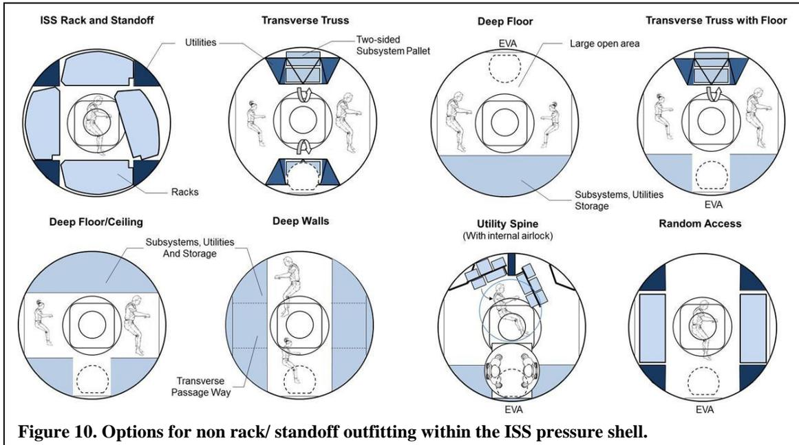
Figure 10. Options for non rack/ standoff outfitting within the ISS pressure shell.
