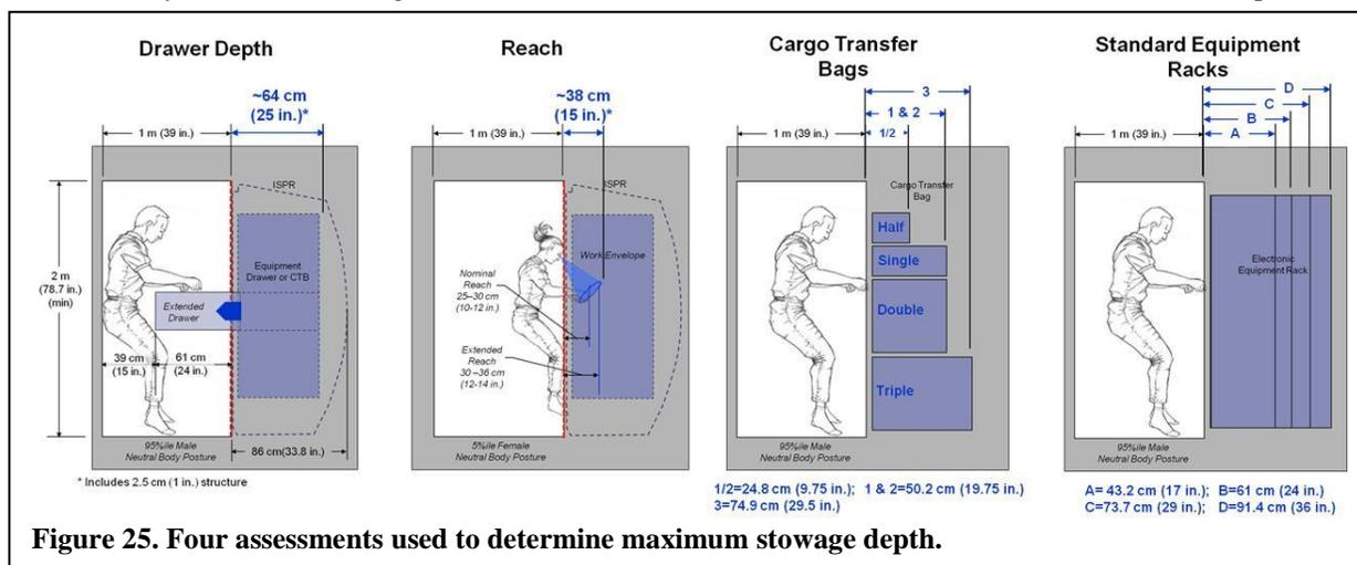
**Figure 25. Four assessments used to determine maximum stowage depth.**
