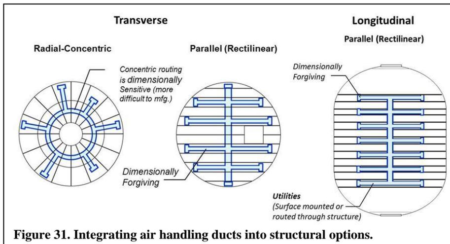
**Figure 31. Integrating air handling ducts into structural options.**
