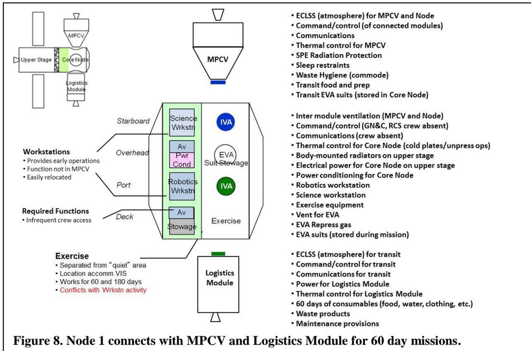
**Figure 8. Node 1 connects with MPCV and Logistics Module for 60 day missions.**
