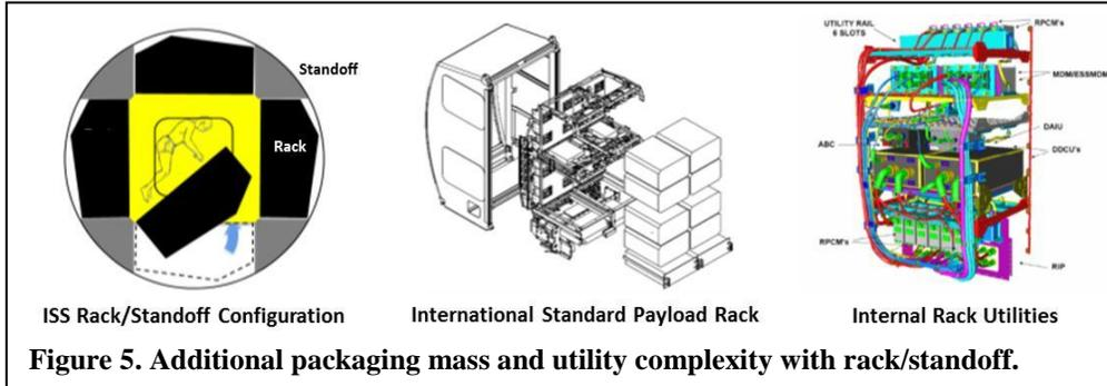
**Figure 5. Additional packaging mass and utility complexity with rack/standoff.**
