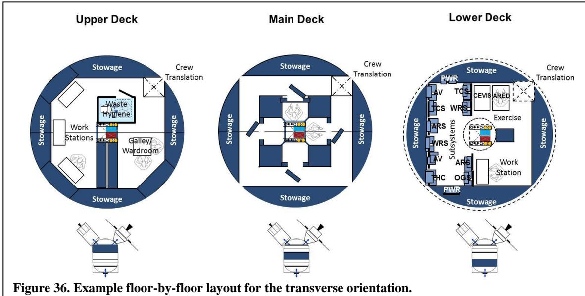
**Figure 36. Example floor-by-floor layout for the transverse orientation.**
