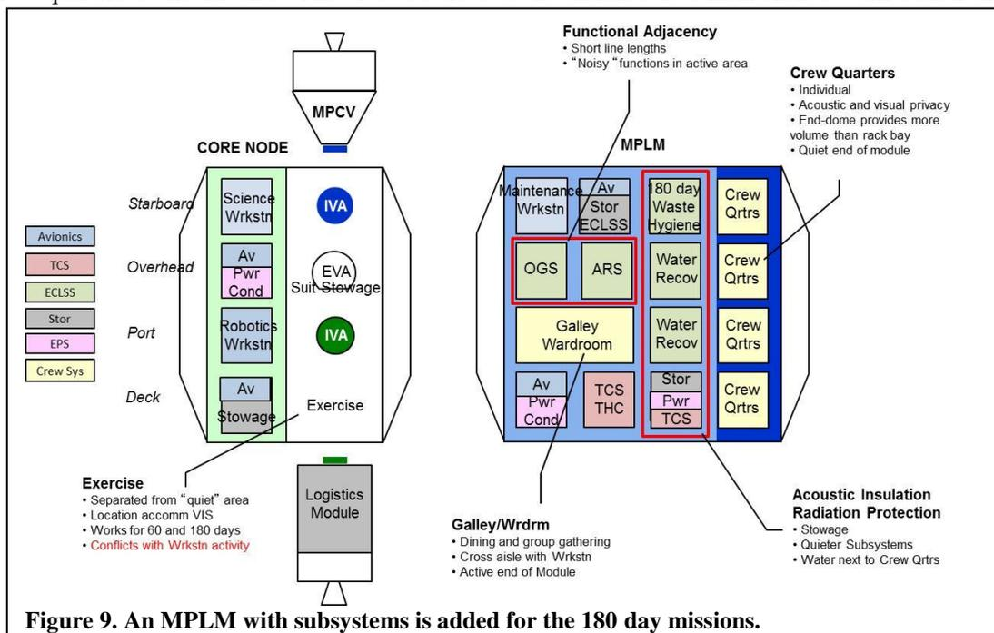
**Figure 9. An MPLM with subsystems is added for the 180 day missions.**
