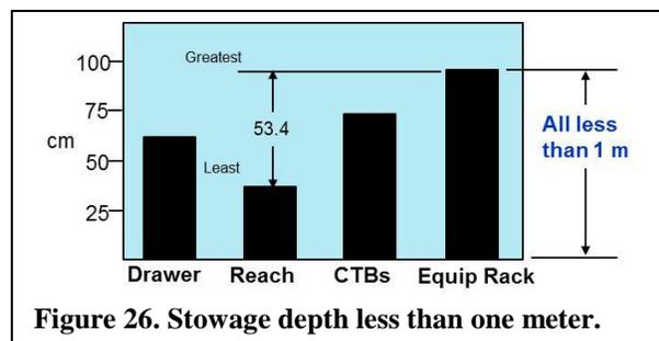
**Figure 26. Stowage depth less than one meter.**
