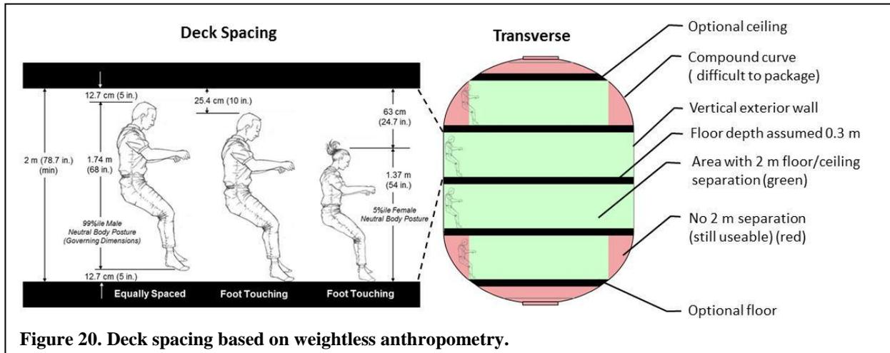
**Figure 20. Deck spacing based on weightless anthropometry.**
