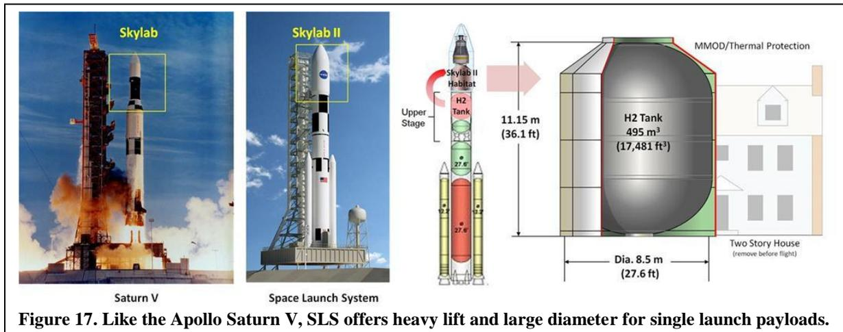
Figure 17. Like the Apollo Saturn V, SLS offers heavy lift and large diameter for single launch payloads.
