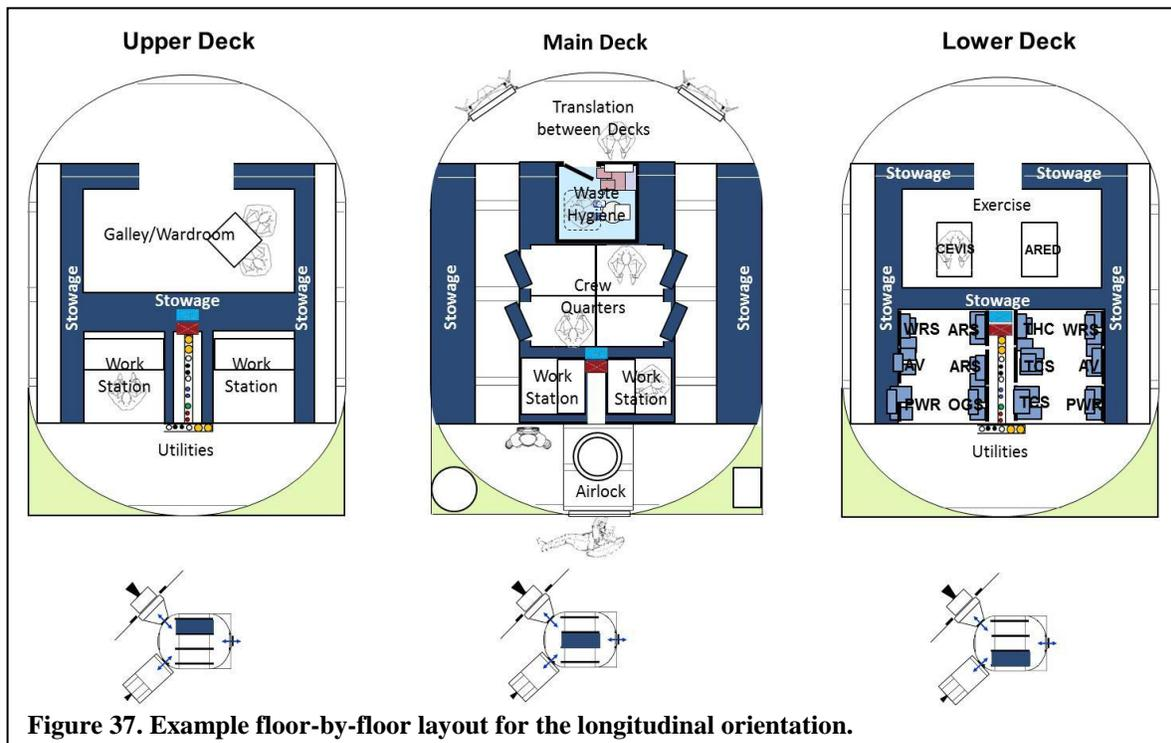
**Figure 37. Example floor-by-floor layout for the longitudinal orientation.**
