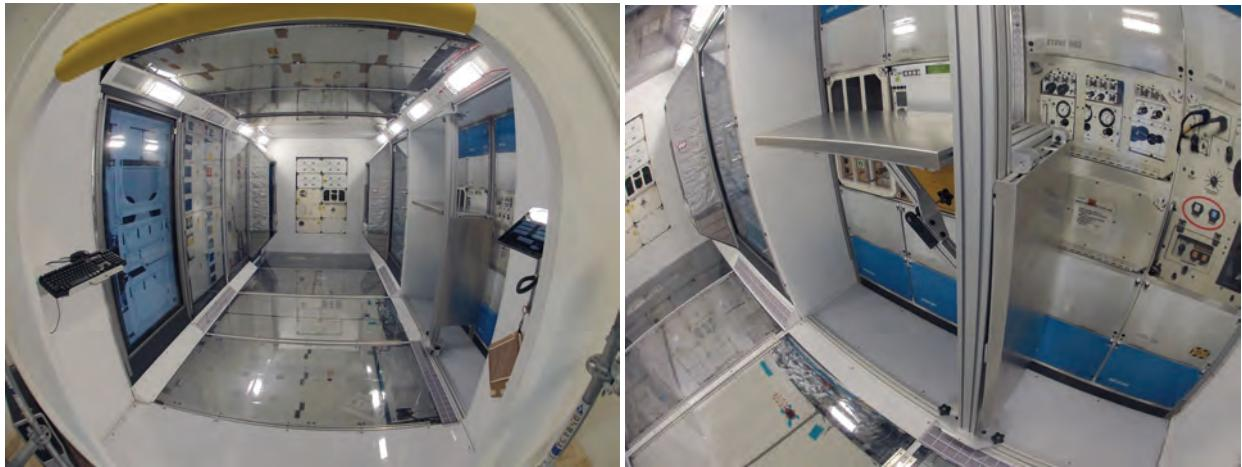
**Figure 20: ISS-derived Cis-lunar Deep Space Habitat Multi-Purpose Logistics Module mockup interior, showing rack front likenesses (left), and Wardroom table mockup**
