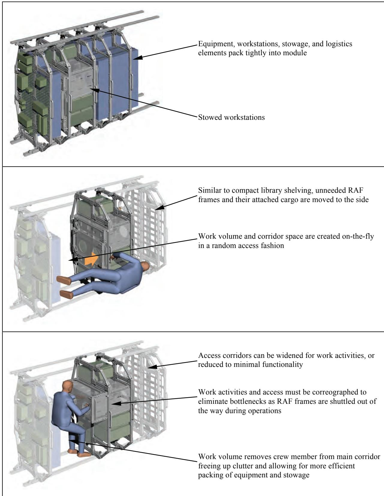
Figure 22: Random Access Frame (RAF) concept (Howe & Polit-Casillas 2014)
