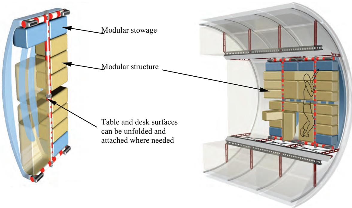
**Figure 16: ISS-derived Cis-lunar Deep Space Habitat Galley / Wardroom concept by Raul Polit-Casillas, Caltech Jet Propulsion Laboratory**
