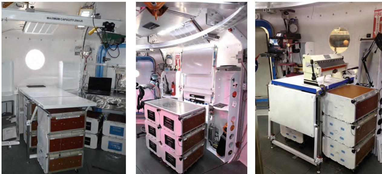
**Figure 7: Habitat Demonstration Unit (HDU) General Maintenance Workstation prototypes – Desert Research and Technology Studies (D-RATS) 2010 (left), D-RATS 2011 (middle), and Mission Operations Test (MOT) 2012 (right)**
