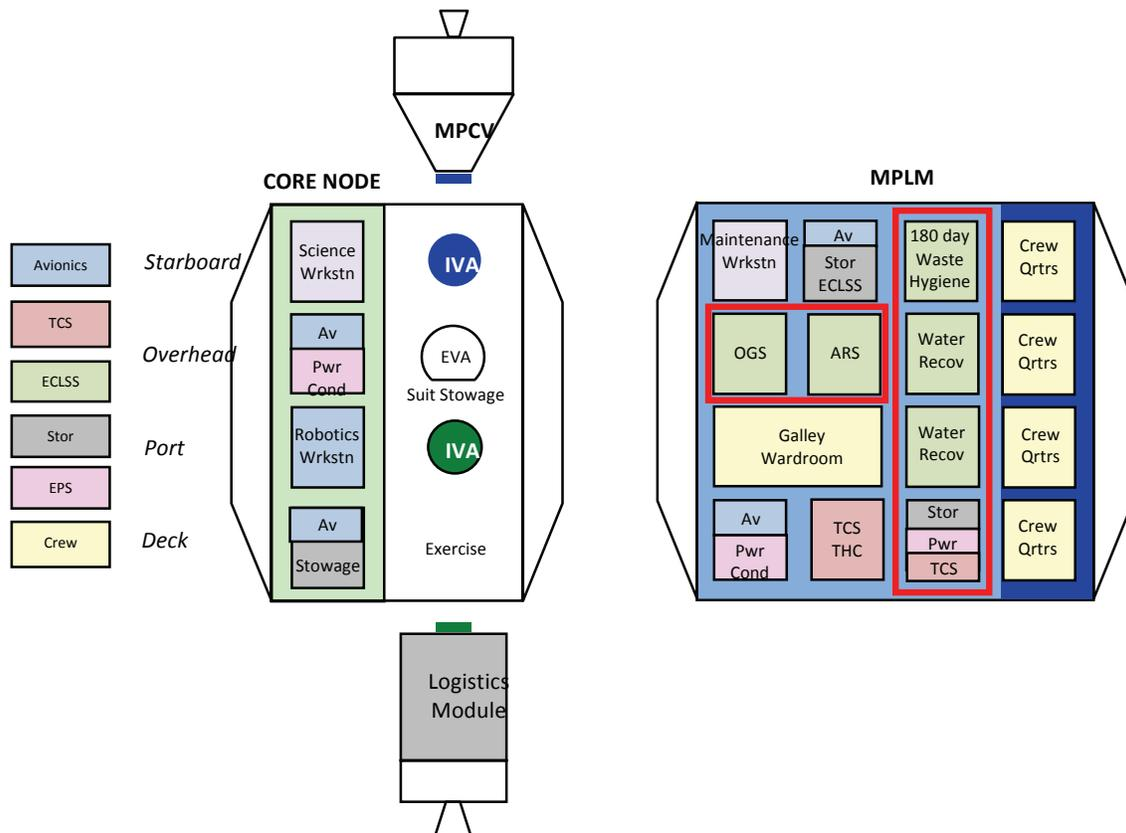
**Figure 4: Cis-lunar Deep Space Habitat 180 day mission layout (courtesy of NASA Marshall Spaceflight Center) – this study covers Telerobotic Workstation in Core Node, and General Maintenance Workstation (GMWS) and Galley / Wardroom in MPLM.**
