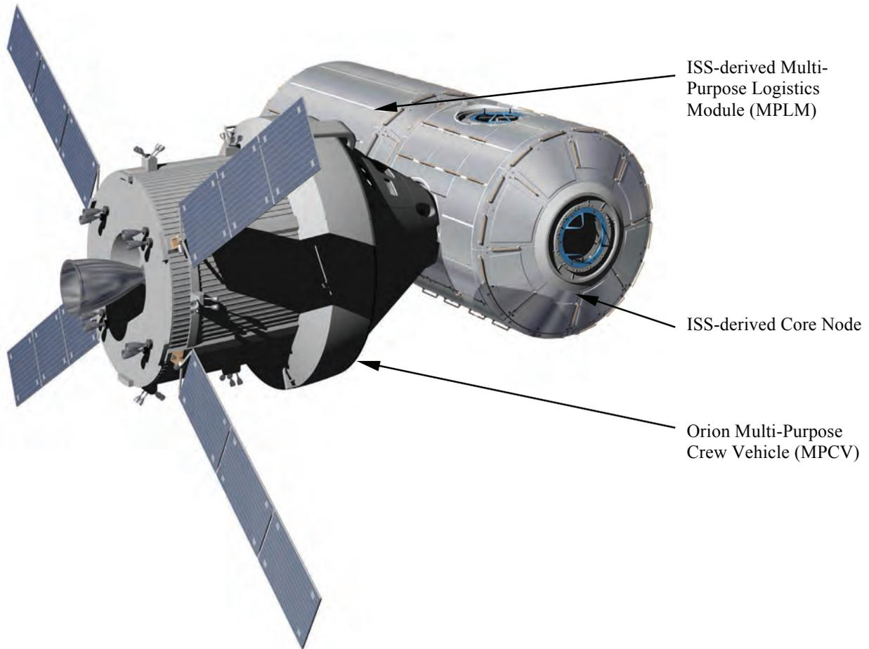
**Figure 2: ISS-derived Cis-lunar Deep Space Habitat with some of the modules needed for a 160-day mission**
