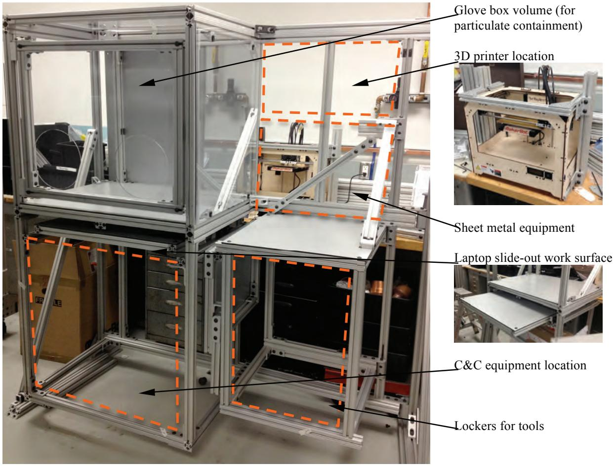
**Figure 25: California Polytechnic University Pomona ISMW prototype work -- testing reconfigurability, deployable, and nesting structures (work in progress)**
