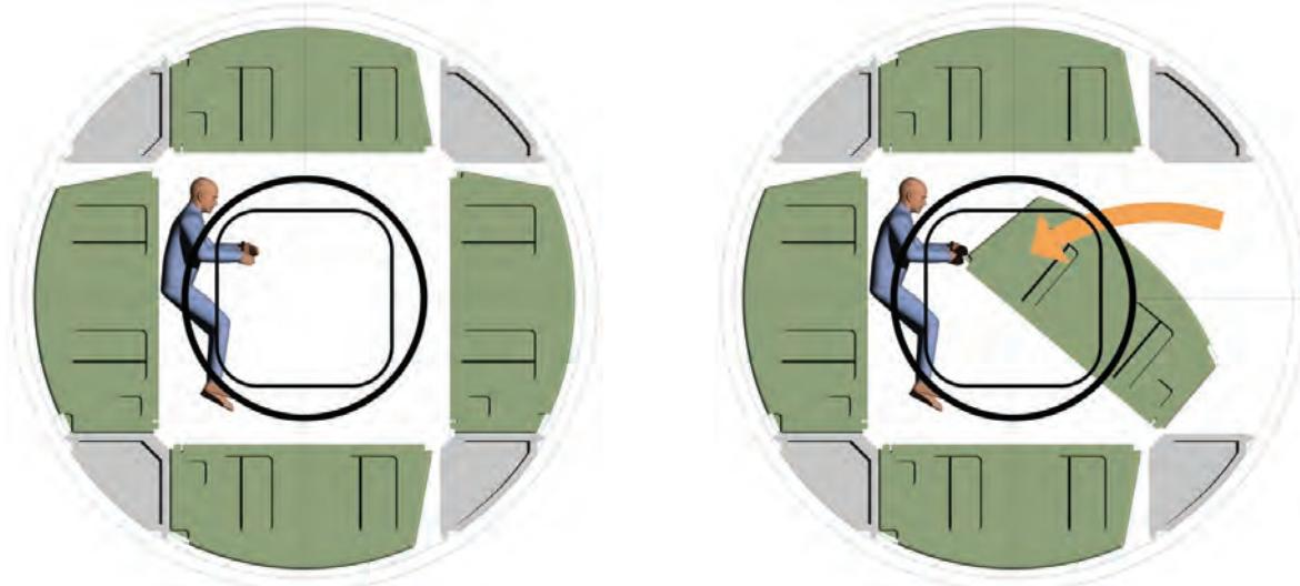
**Figure 1: Cross-section of ISS modules showing the International Standard Payload Rack (ISPR) method of organizing equipment and logistics (left, shown as green modules attached to gray standoff structure) – rack modules can be swapped in and out with frequent resupply (right)**
