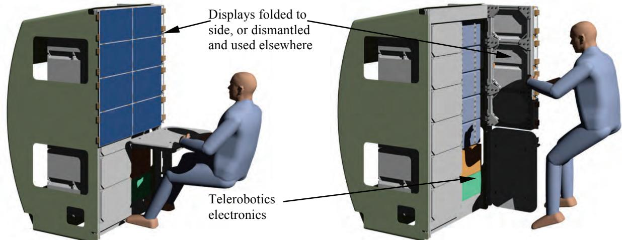
**Figure 14: Rack-based Telerobotics Workstation, single-bank tiled video wall (left), and CTB stowage volume behind (right)**
