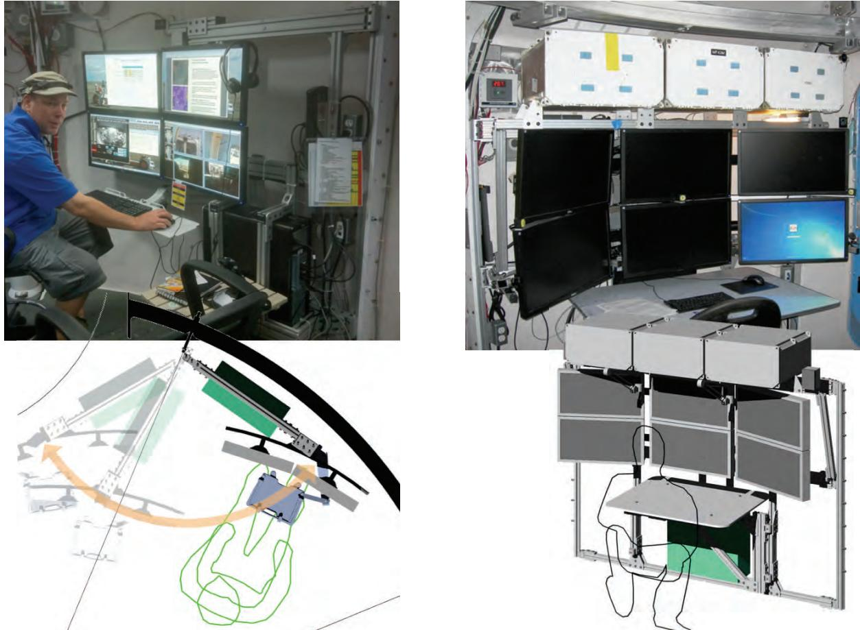
**Figure 11: Habitat Demonstration Unit (HDU) Telerobotics & IVA Workstation prototypes – Desert Research and Technology Studies (D-RATS) 2010 swing-away design (left), and D-RATS 2011 deployable workstation version (right)**
