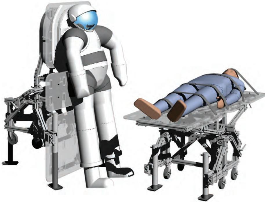
**Figure 6: Alternative multi-orientation uses for re-deployable work surfaces in an earth-analog environment**
