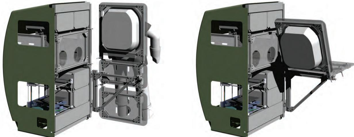
**Figure 10: Rack-based GMWS in suit maintenance configuration (left), and Personal Life Support System (PLSS) adjustable maintenance configuration**
