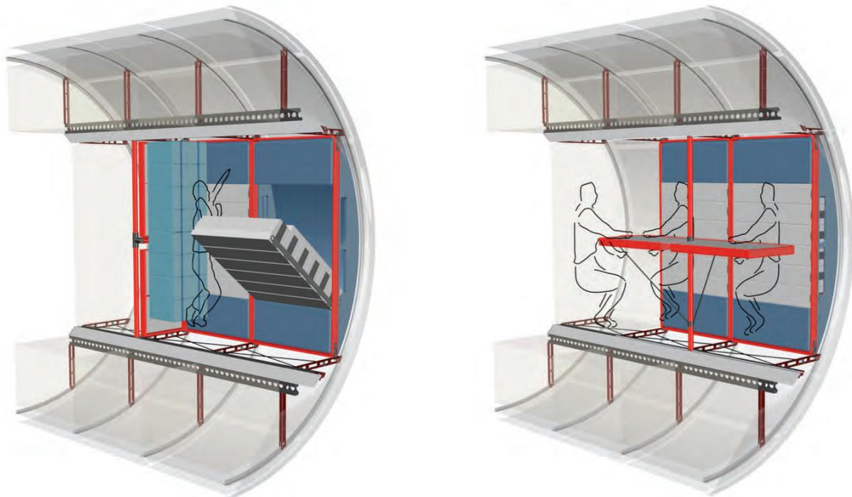
Figure 17: Galley / Wardroom storage pallets (left), and deployable table (right) (courtesy Raul Polit-Casillas, Caltech Jet Propulsion Laboratory)
