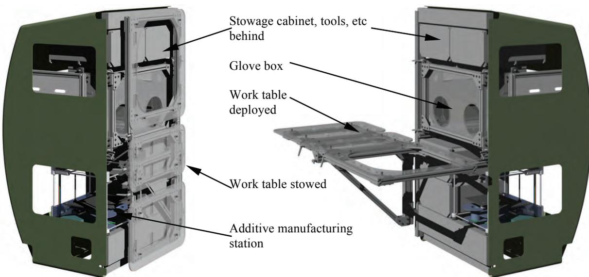
**Figure 8: Rack-based General Maintenance Workstation (GMWS) design, stowed (left), and with horizontal work surface deployed (right)**
