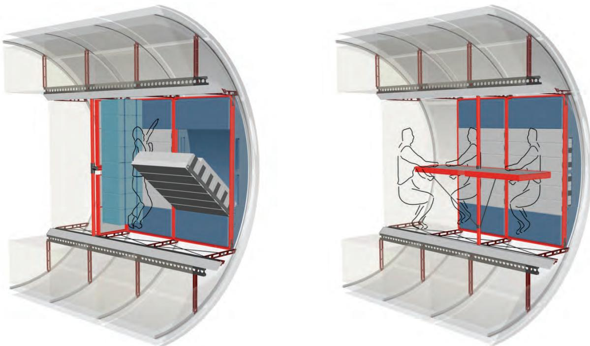
**Figure 17: Galley / Wardroom stowage pallets (left), and deployable table (right) (courtesy Raul Polit-Casillas, Caltech Jet Propulsion Laboratory)**
