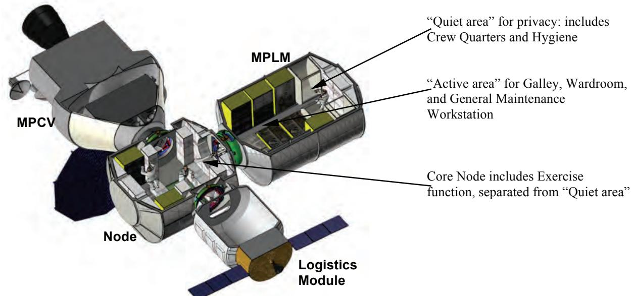
Figure 3: Cis-lunar Deep Space Habitat section (courtesy of NASA Marshall Spaceflight Center)
