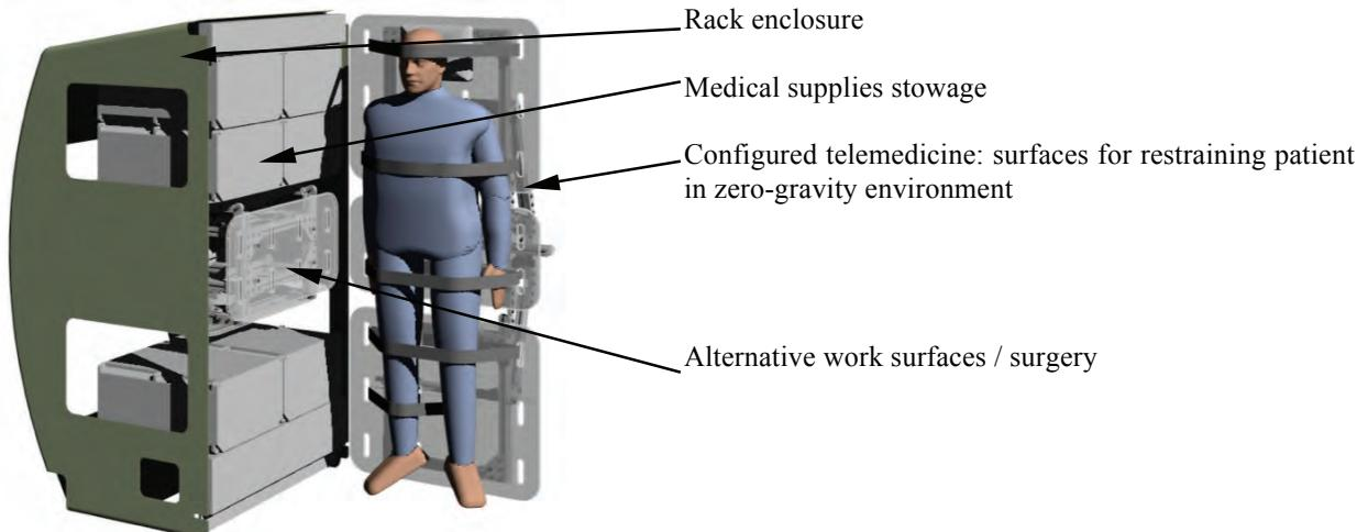
**Figure 21: Using articulated folding work surfaces, a variety of functions can be accommodated, such as telemedicine workstation**
