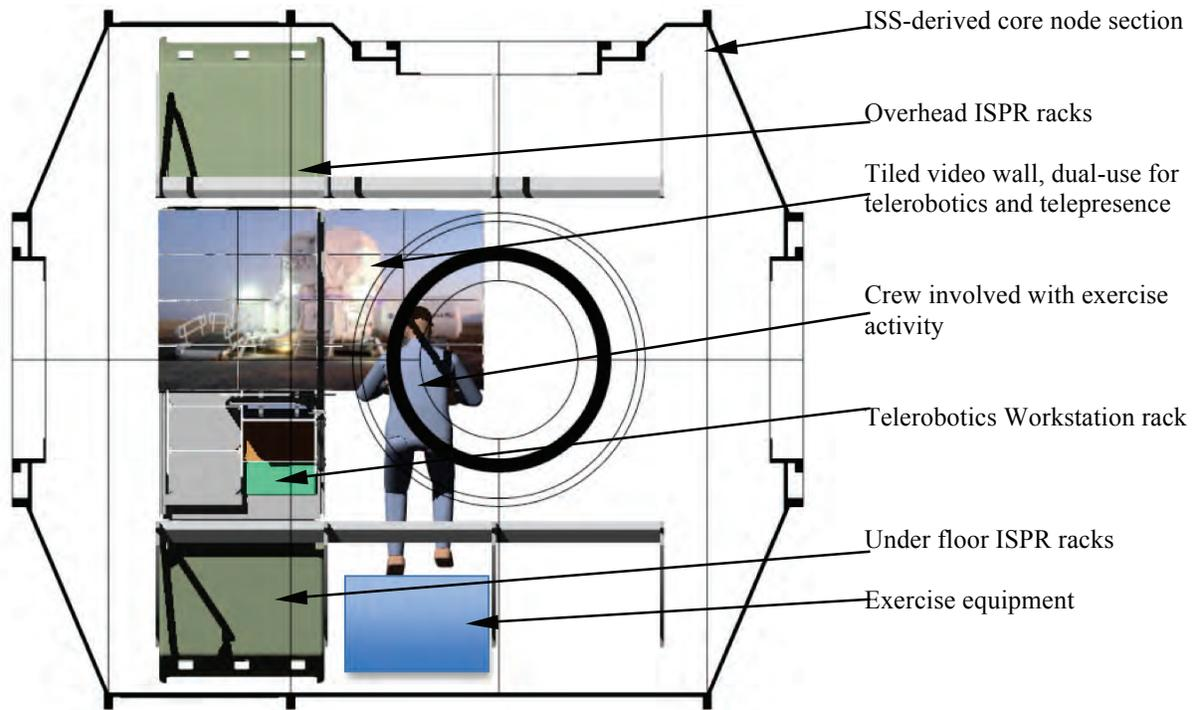
Figure 12: ISS-derived Cis-lunar Deep Space Habitat Telerobotics Workstation concept
