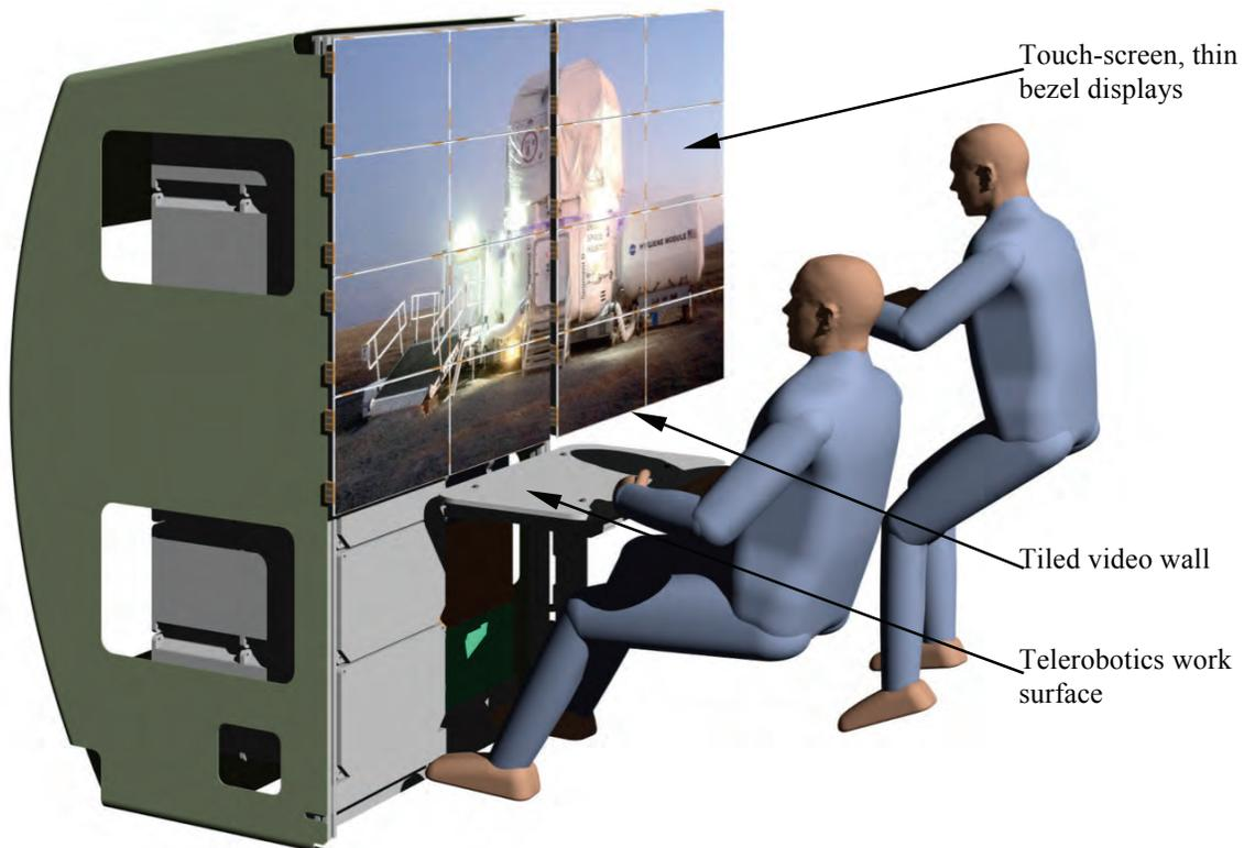
Figure 13: Rack-based Telerobotics Workstation concept with double-bank tiled video wall
