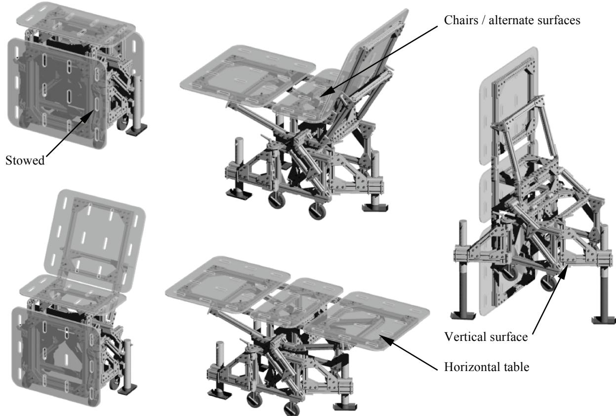
**Figure 5: Modular deployable work surfaces study, exploring multi-fold, articulated, clamping surfaces for a variety of orientations**
