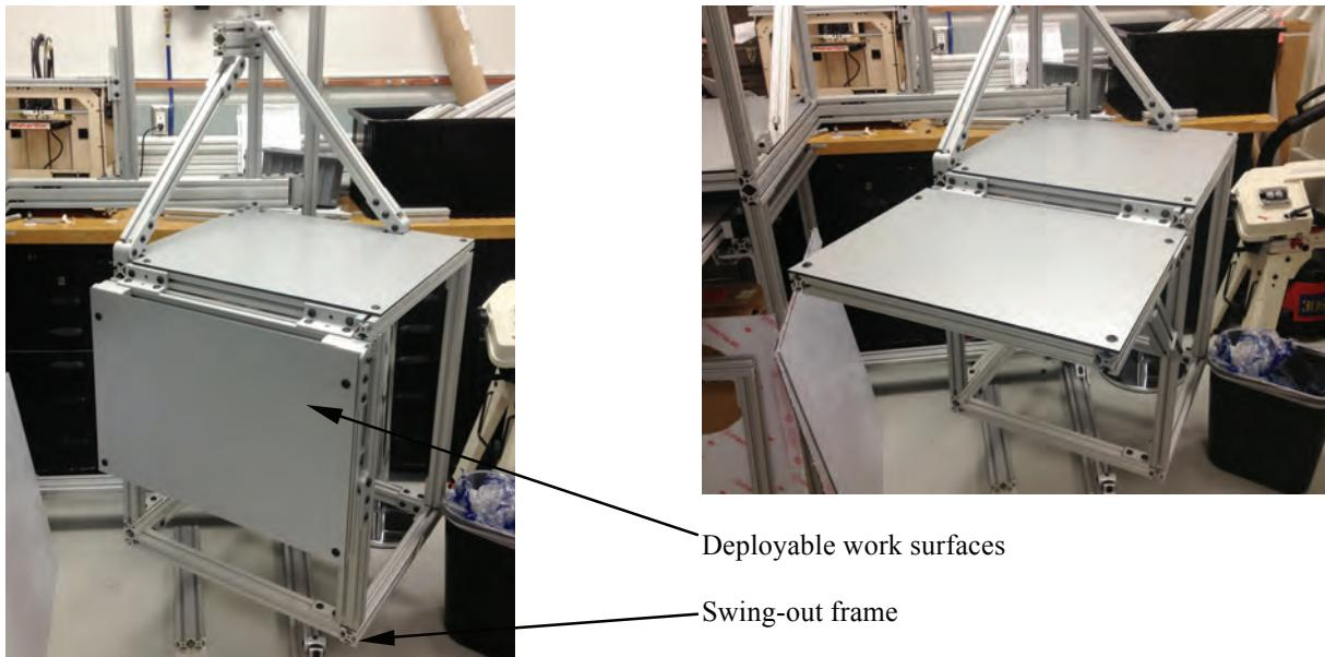
**Figure 26: California Polytechnic University Pomona ISMW prototype work -- testing reconfigurability, deployable, and nesting structures (work in progress)**
