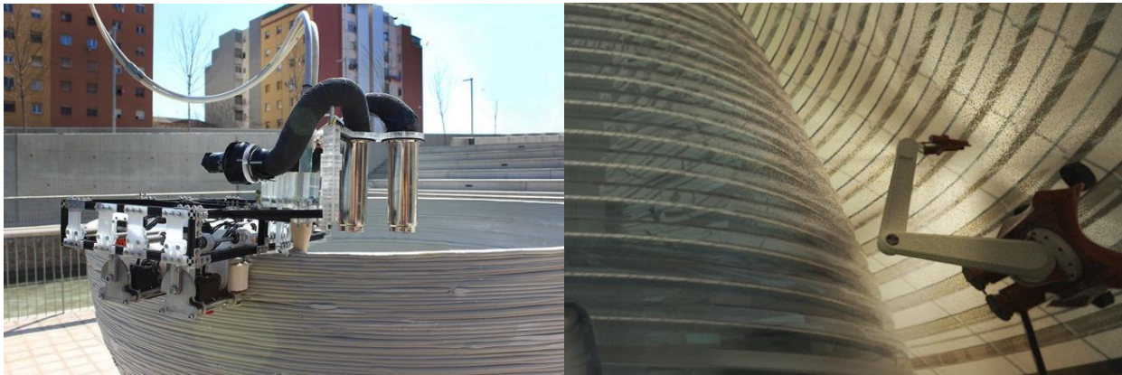
Figure 10. (Left) “Minibuilders” construct and simultaneously climb a wall at the IAAC was the basis for the (Right) Mars Ice House concept image of a robot capable of scaling the wall it has already constructed.
