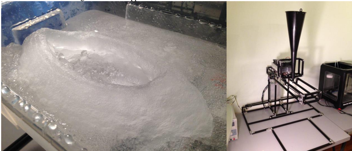
Figure 11B. (Left) Additive deposition of water ice, constructed by Petr Novikov for SEArc. (Right) water ice deposition mechanism showing movement in multiple axes.
