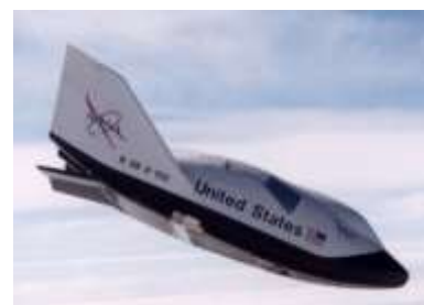
Figure 2. X-38 Lifting Body Reentry Vehicle By NASA/Carla Thomas – Armstrong Photo Gallery
