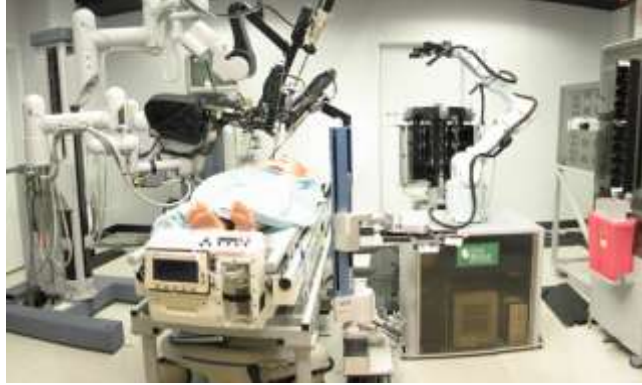
Figure 3. The SRI-led Trauma Pod, developed for DARPA as a next-generation mobile robotic surgery platform for the military
