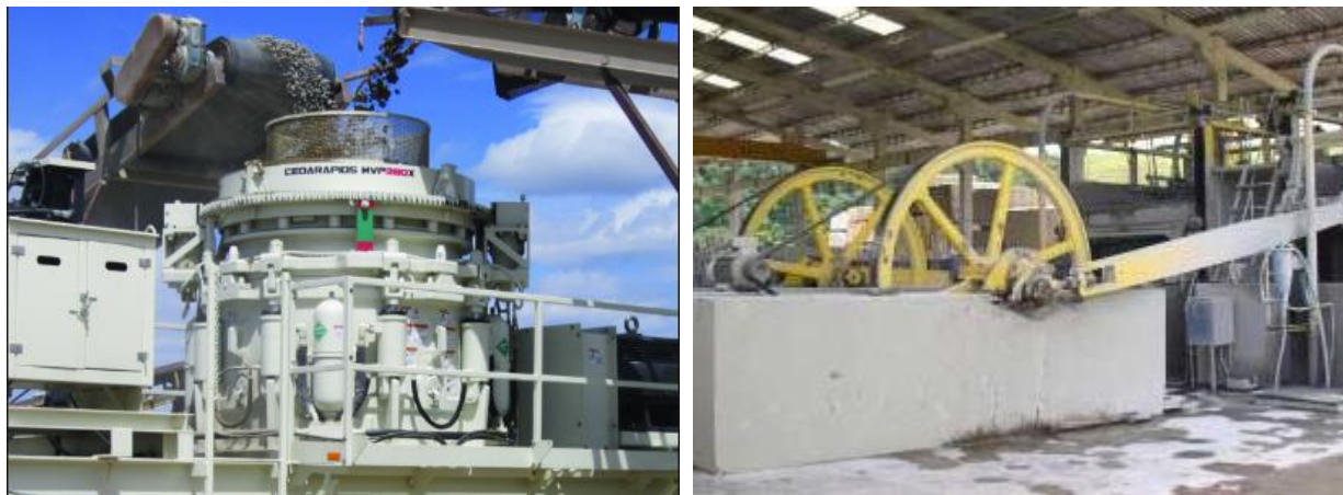
Figure 4a, b – 4a shows a cone crusher crushing rocks into finer materials (“P&Q”). 4b shows a slab cutter at work in the quarry (“Quarry”). Large slabs cut from lunar basalt could be used to pave landing pads and roads, and to build dustfree platforms on which habitats and other structures may be erected.
