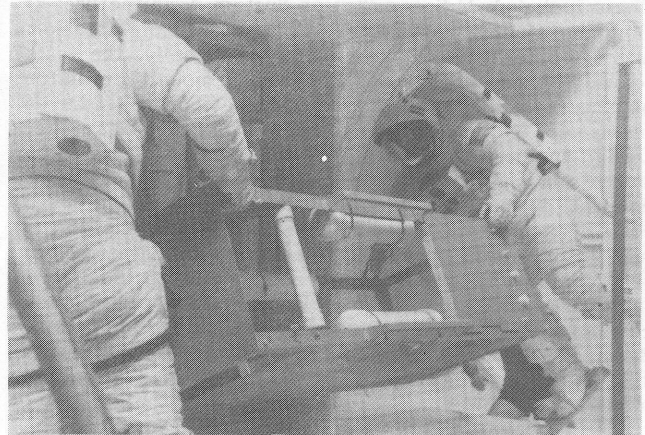
Figure 4 Test Subject Removes Equipment Rack to Provide Access to Damaged Shell
