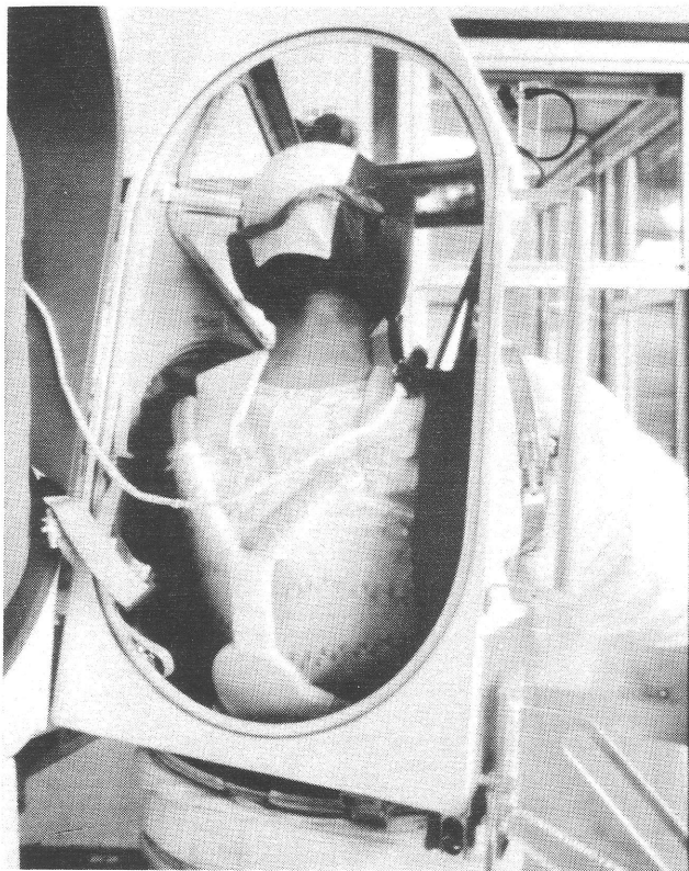
Figure 5 The rear entry of the CCPS engineering test article accommodates modular backpack options.
