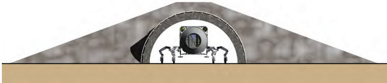
Figure 9: Habitat would be carried into unpressurized garage via ATHLETE mobility system
