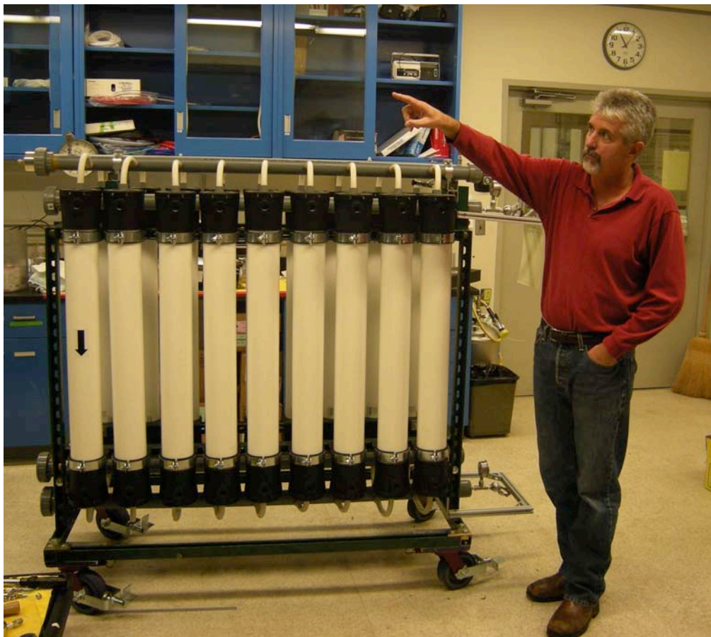
FIGURE 4. Michael Flynn with the FO urine and gray-water processing array for the NASA Ames Sustainability Center, set up for testing in the Bioengineering Branch life support lab.
