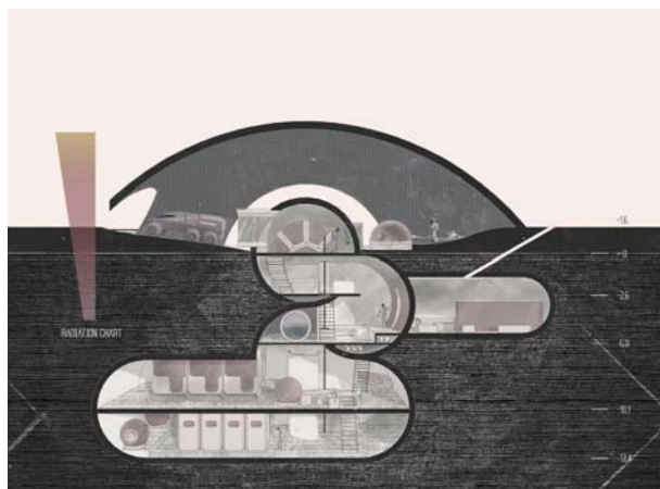
Fig. 8. Section of the astronaut training centre, showing the work and living areas. (credit: HB2, TU Wien, Design Studio Moon Village, Dogan, Oblitcova, 2018)
