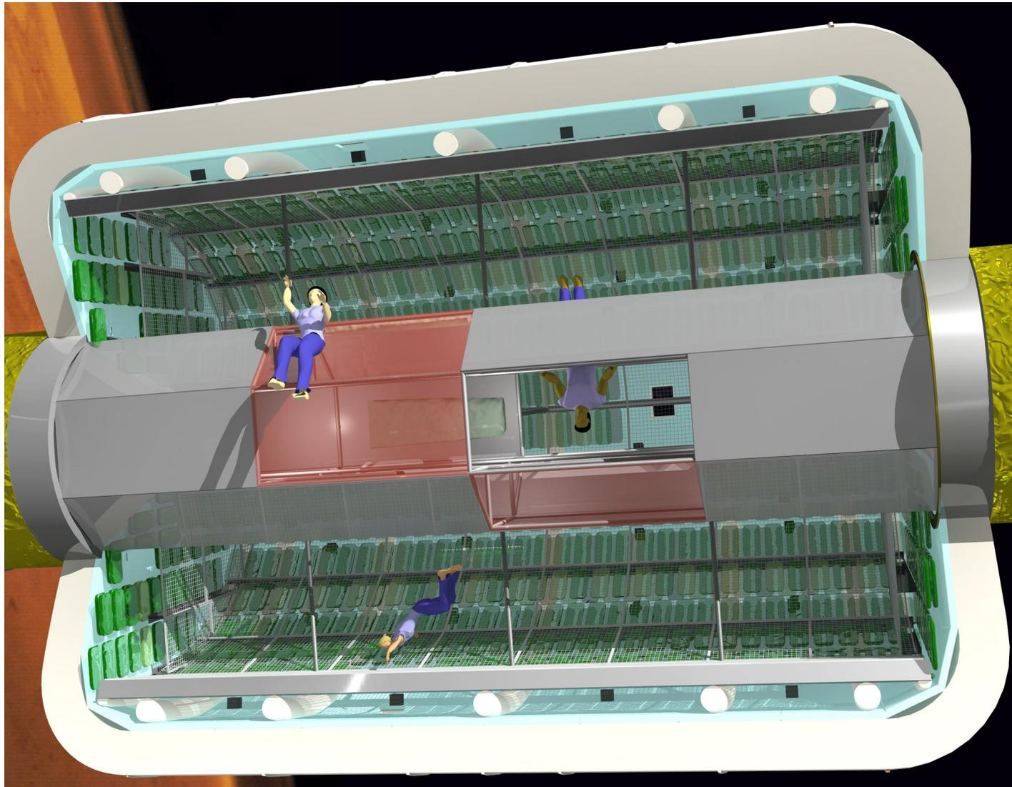
FIGURE 15. Enlarged view of the longitudinal section (from FIG. 1) through a Bigelow 330 (TransHab type) space habitat, showing a detailed view of two layers of Air Revitalization Bags installed around the inside perimeter and end walls of the inflatable pressure vessel. Drawing Credit: François Lévy.
