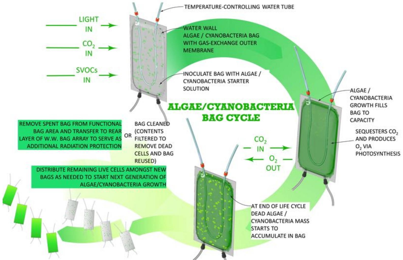
FIGURE 11. Air Revitalization Subsystem -- Algae Growth/Cyanobacteria Growth Cycle.
