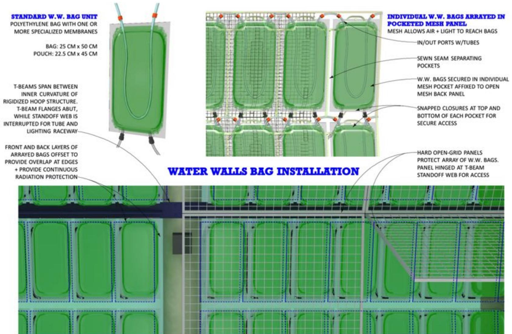
FIGURE 12. Installation of the Air Revitalization / Algae Growth Subsystem in a Habitable Space Module.
