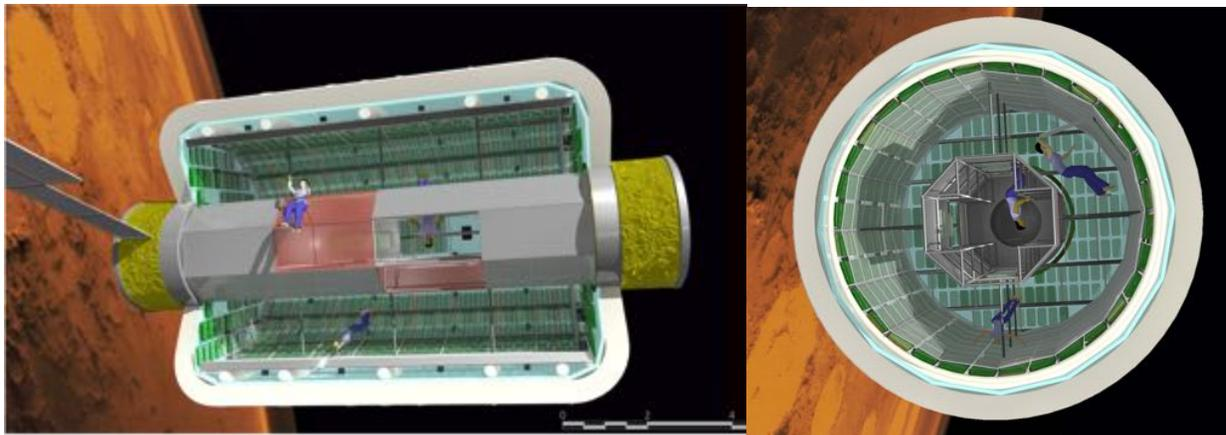
FIGURE 1. Longitudinal and transverse section views of a “TransHab” type space habitat inflatable module showing the Water Walls ECLSS system lining its inner Walls. Credit: François Levy.
