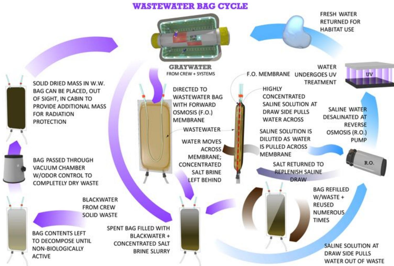
FIGURE 13. Blackwater/Solids Processing Subsystem in the Wastewater Treatment Cycle. Design Credit: Renée L. Matossian.
