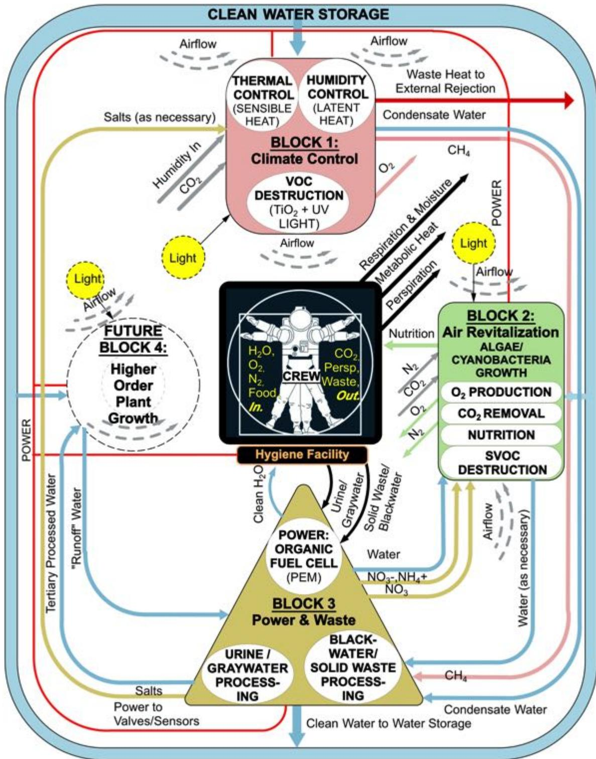
FIGURE 5. Process Block Diagram shows the three fundamental process blocks and the placeholder in Block 4 for future higher order plants for food crops. Credit: Renée L. Matossian, Marc M. Cohen.
