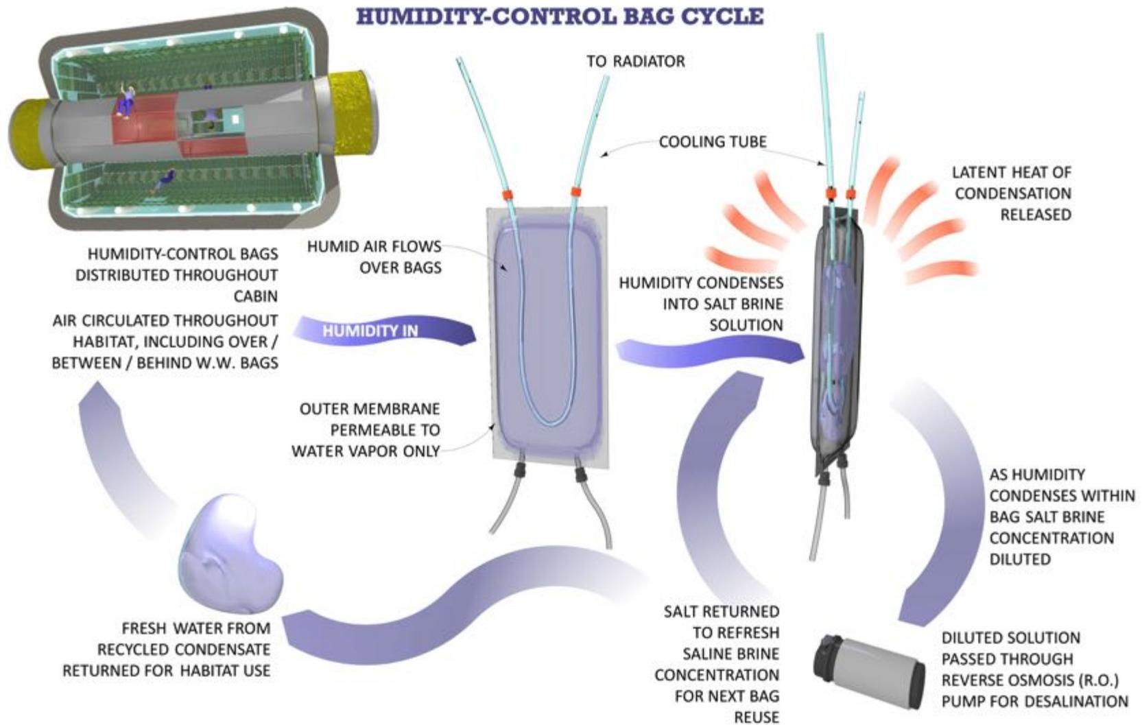
FIGURE 10. Humidity Control Subsystem – Humidity Control Bag Cycle within the Climate Control Process Block.
