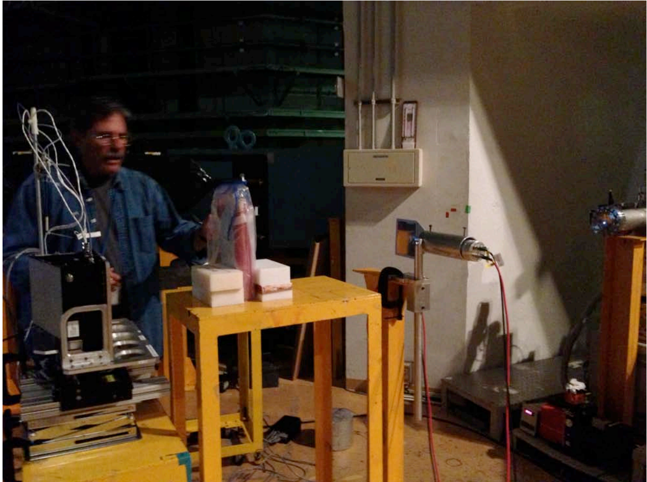
FIGURE 6. Detection system for the 230 MeV/nucleon ^4\text{He} tests. Here the beam direction goes from right to left. The beam passes through the trigger scintillator, two forward osmosis bags and the CRaTER instrument at the left of the frame.
