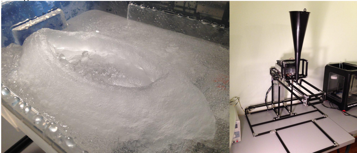
Figure 6B. (Left) Additive deposition of water ice, constructed by Petr Novikov for SEArc. (Right) water ice deposition mechanism showing movement in multiple axes.
