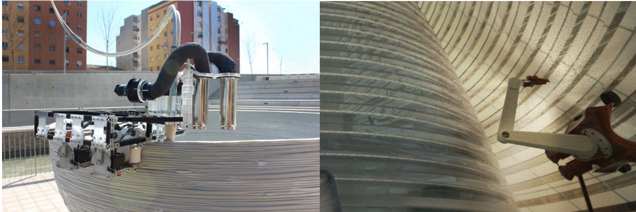
Figure 5. (Left) “Minibuilders” construct and simultaneously climb a wall at the IAAC was the basis for the (Right) Mars Ice House concept image of a robot capable of scaling the wall it has already constructed.
