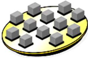
Fig. 13 Micro nano-tower solar array towers are 100 microns tall, 40 microns square, and separated by 10 microns
