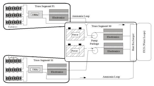
Figure 4.4.3 Active thermal control system hardware for ISS at Assembly Complete. As noted by the arrows, ammonia flows from radiators to the common ITCS/EATCS heat exchanger then to the warmer thermal loads associated with electronics mounted on coldplates. Each Thermal Radiator Rotary Joint (TRRJ) rotates to position the radiator panels so that they face anti-Sun, or "edge-on" to the Sun. The bulk of the EATCS is located on truss segments S0, S1, and P1.
