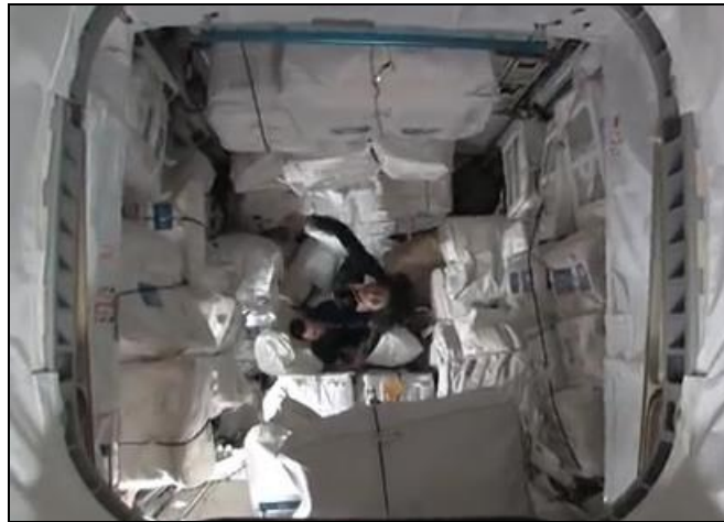
The Leonardo Permanent Multipurpose Module, installed in March 2011, is used for storage on the ISS.
