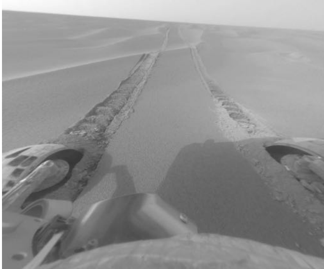
Figure 4. Image taken on Sol 482 from the front hazard camera onboard the Mars Exploration Rover Opportunity. The rover was mired in soft dune material which severely limited the rover's mobility.
