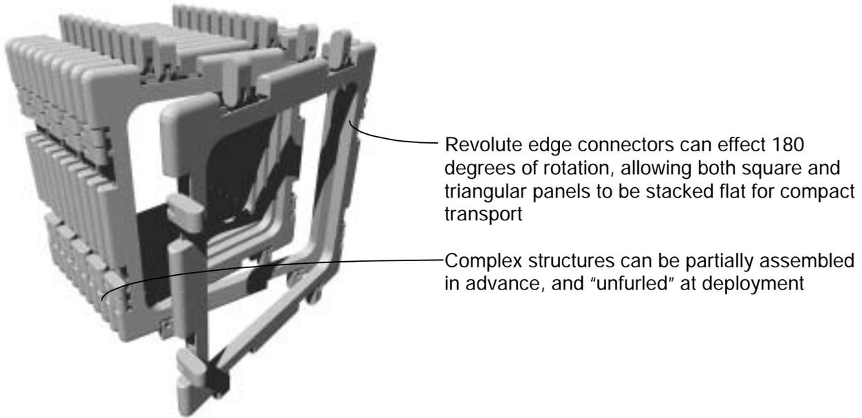
**Figure 9: Stackable trigon panels**
