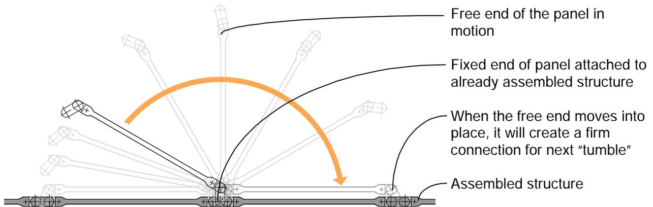
Figure 6: Trigon panels "tumble" along existing structure
