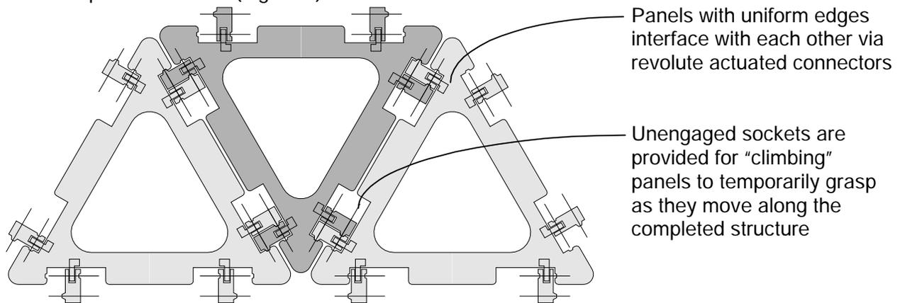
Figure 5: Trigon connection: engaging each other at edges
