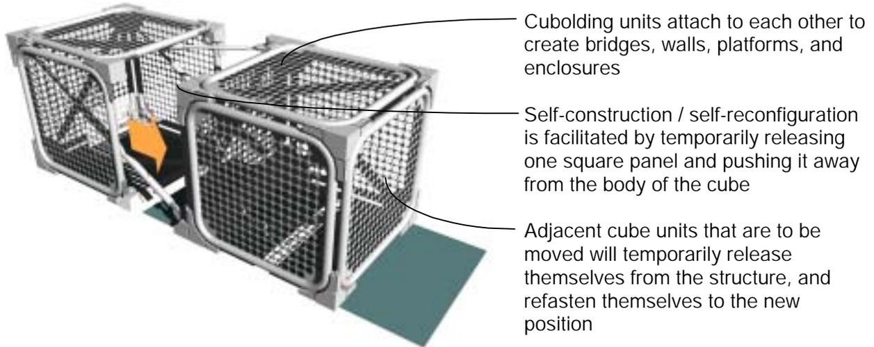
Figure 3: Relocating cube structure units
