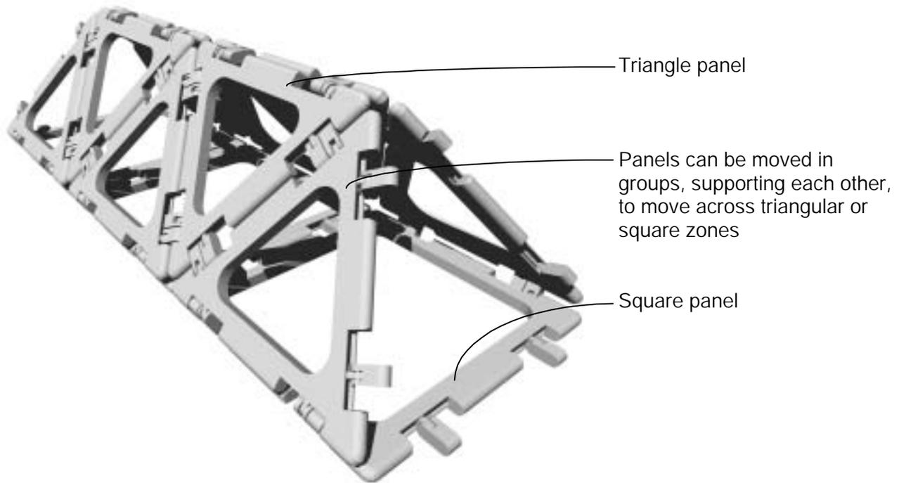
**Figure 8: Trigon truss structures**
