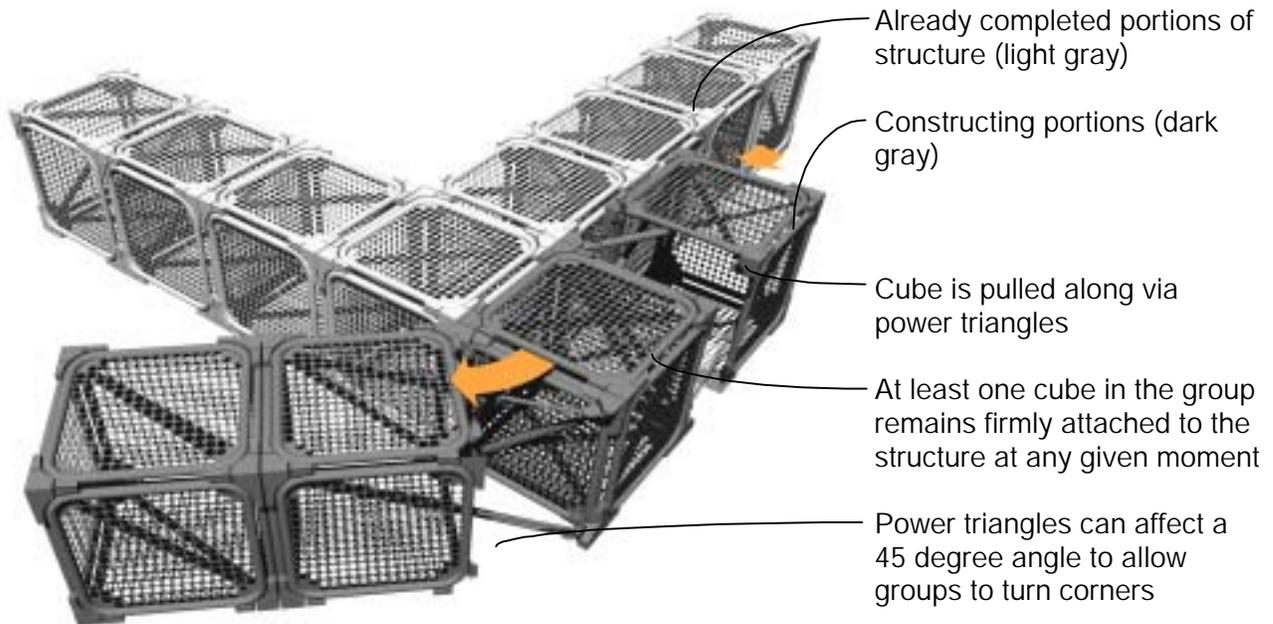
Figure 4: Cube scaffolding units can climb and turn corners
