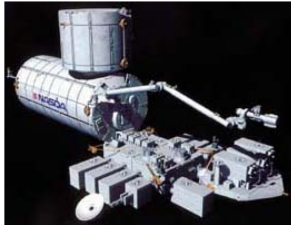
Figure C.2-3. The Japanese Experiment Module with its associated Exposed Facility and Remote Manipulator System. (Image courtesy of NASDA)
