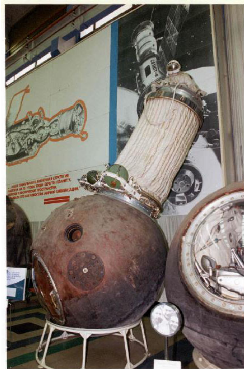
Figure B.4-1. The Voskhod spacecraft (minus the service module) with the inflatable airlock deployed. Note head and shoulders of a suited crewmember at the top of the airlock. (Photo courtesy R. Fullerton)
