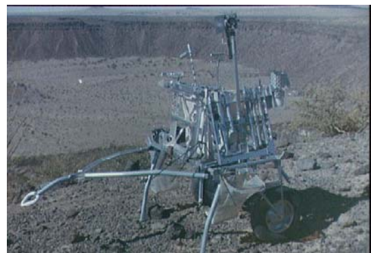
Figure B.3-5. The Apollo 14 astronauts used this prototype of the MET during their geological and lunar surface simulation training in the Pinacate volcanic area of northwestern Sonora, Mexico. (NASA photo S70-29505).
