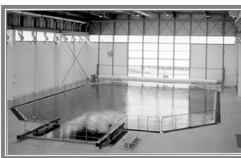
Figure C.4-3. The octagon-shaped neutral buoyancy facility pool. The preparation platform is in foreground and rolled up pool cover in background. (Photo courtesy of ESA)
