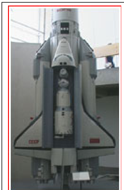
Figure B.4-4. A model of the Buran space shuttle. The airlock is located at the upper end of the payload bay.
