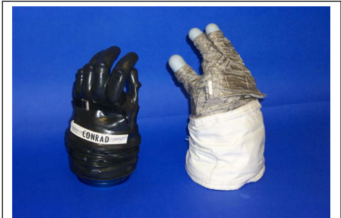
Figure B.1-6. Apollo EVA glove assembly. (Photo courtesy S. Hoffman).
