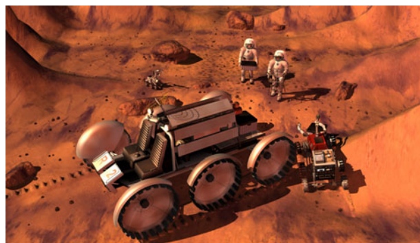
Figure E-5. One example of an unpressurized rover capable of carrying two crew and additional equipment. (NASA image)
