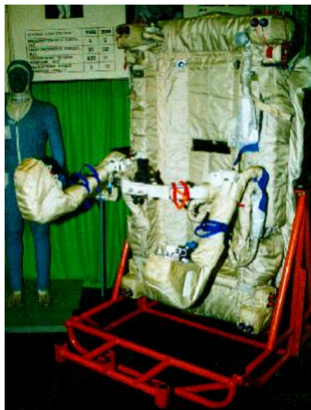
Figure B.1-10. The SPK maneuvering unit, designed for use with the Orlan-DMA suit.
