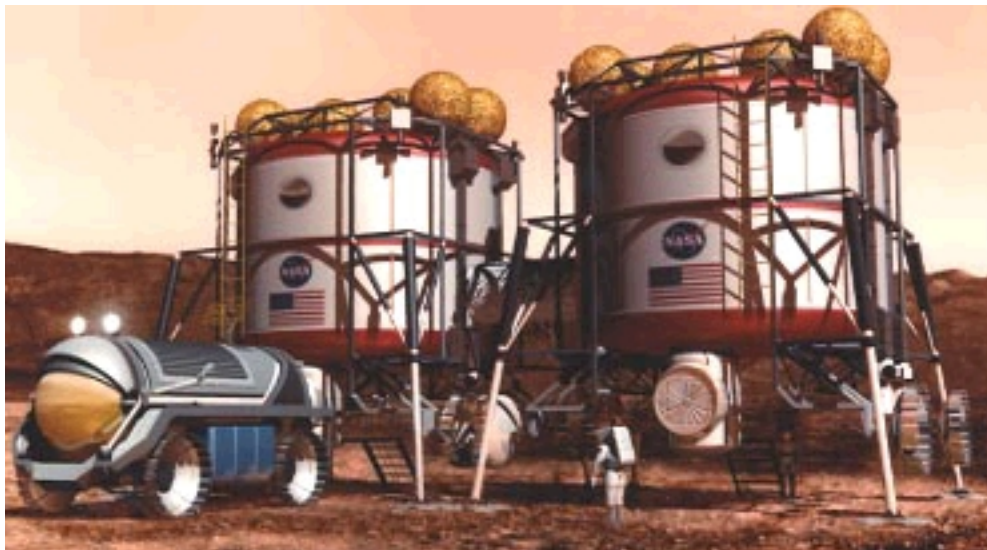
FIGURE 2 This rendering by John Frassanito of the Pressurized Rover docking to the First Mars Habitat is the quintessential image of the rover as a component of mission architecture. Note the airlock nodules that hang down below the habitat cylinders, to put them on a level with the rover docking port and to place them closer to the ground for EVA astronauts to descend the stair-ladder on foot. The front end of the rover resembles a giant space suit helmet facemask with metallized lens and swing-down visors (Courtesy NASA Johnson Space Center, 1993)
