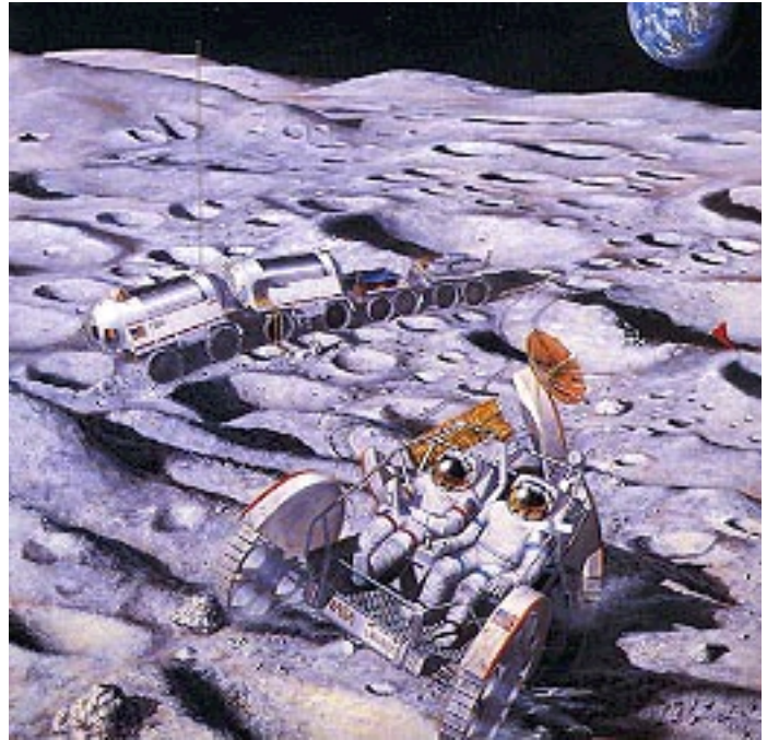
FIGURE 3. Eagle Engineering Study for a Lunar Surface Transportation Rover for NASA -Johnson Space Center (1988) which would carry unpressurized rovers with it. (Courtesy of NASA-Johnson Space Center).
