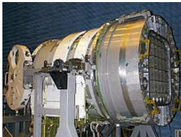
FIGURE10 Kibo (JEM) Scientific Airlock assembly . Note the round inner hatch swung open to the left, and the square outer hatch closed on the right. (Photo courtesy of NASDA, 1999).
