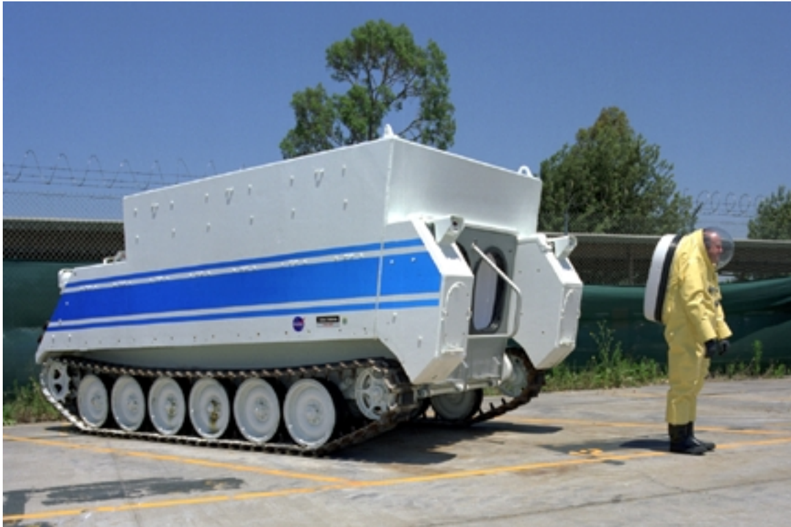
FIGURE 5. Rear oblique view of the HazMat vehicle showing the Suitport inner hatch in the aft bulkhead and the Suitport/ Portable Life Support System (PLSS) modification to the rubber HazMat suit.
