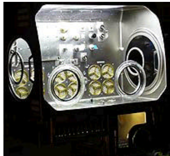
FIGURE 3. Microgravity Science Glovebox for Space Station, (Courtesy NASA-Marshall Space Flight Center).
