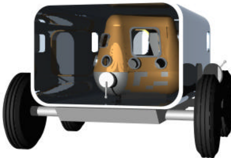
FIGURE 11. Rear view of a simplified planetary rover, with the aft bulkhead removed. The scientific sample airlock appears on the starboard (right) side, between the two wheels, with its handle projecting up at about 45°. The sample airlock's internal hatch opens into the Astrobiology glovebox. The sample exit airlock appears in the center of the rover cabin, with its handle pointing straight down.
