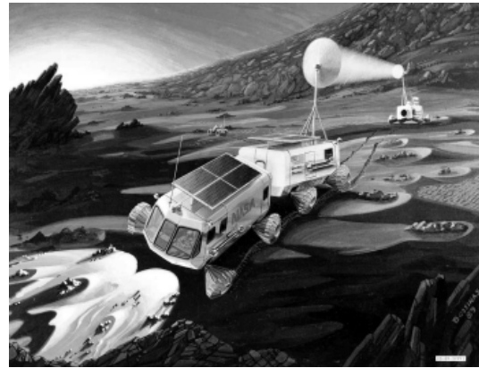
Figure 3. Robert Cataldo's concept for a "follower" nuclear reactor rover. Courtesy of Robert Cataldo, NASA-Glenn Research Center.
