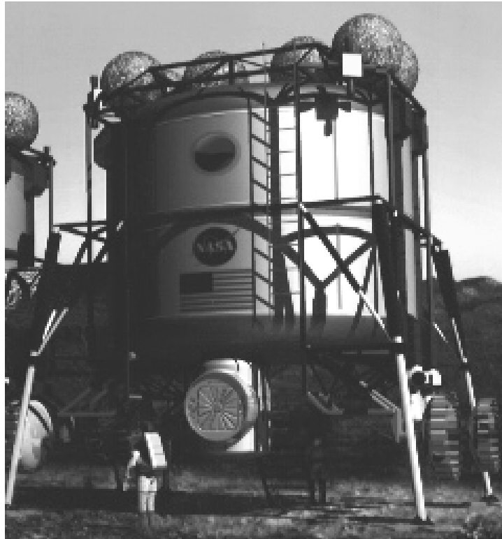
Figure 1. Pre-integrated, hard pressure vessel habitat. Concept by Kent Joosten at Johnson Space Center, courtesy of Kriss Kennedy, NASA Johnson Space Center
