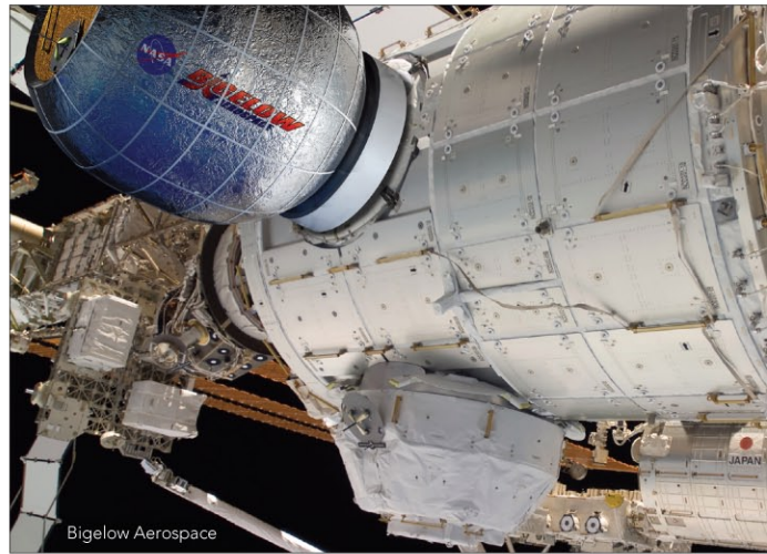
An artist’s rendering shows the Bigelow Expandable Activity Module attached to the International Space Station.
