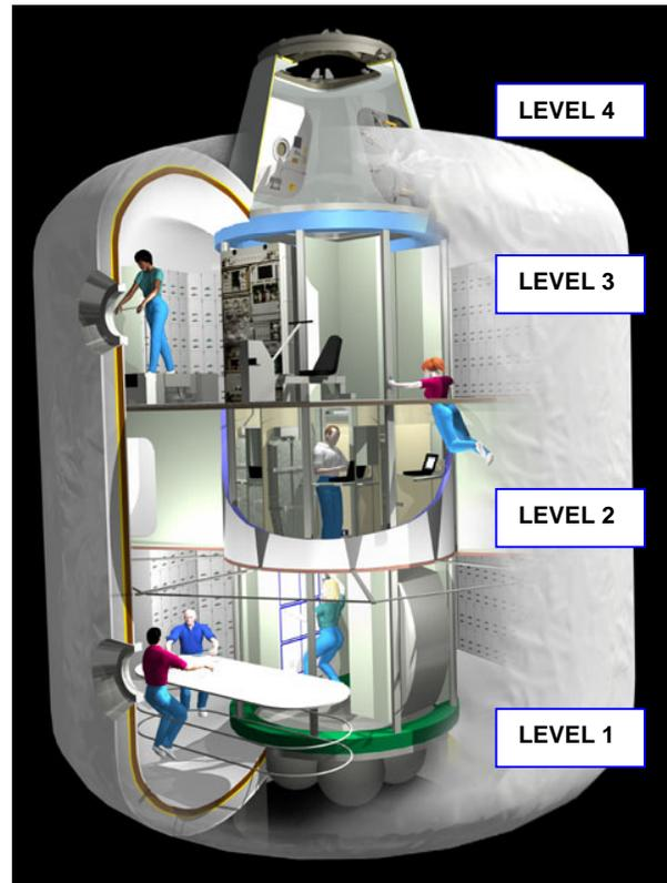
Figure 2. ISS TransHab Internal View
