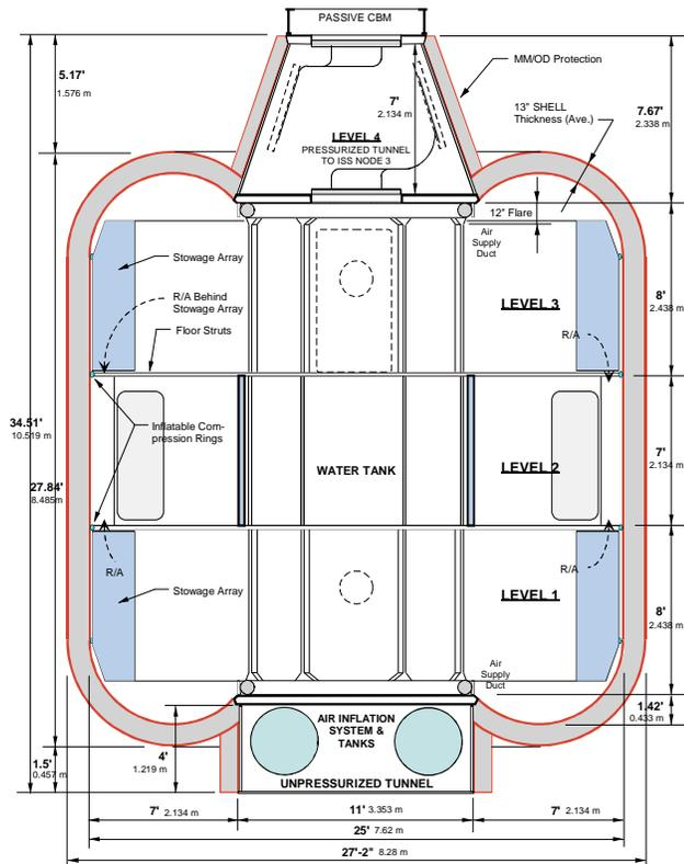
Figure 1. ISS TransHab Section
