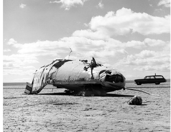
Figure 25: Crash of M2F2 test vehicle
