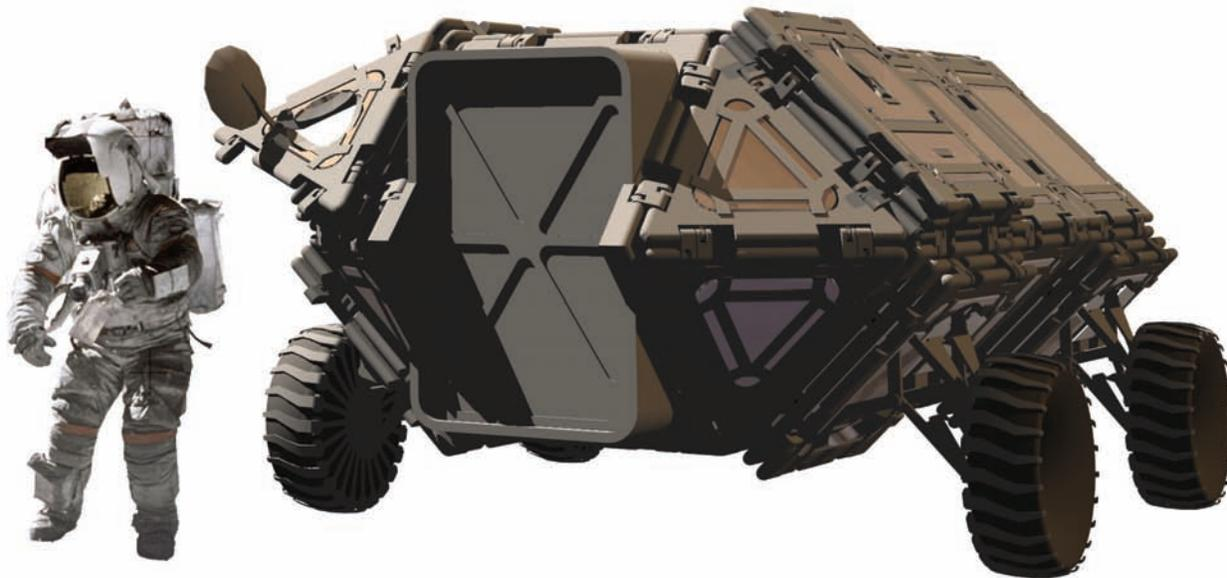
**Figure 15: Pressurized rover constructed of Trigon panels and inflatable liner**
