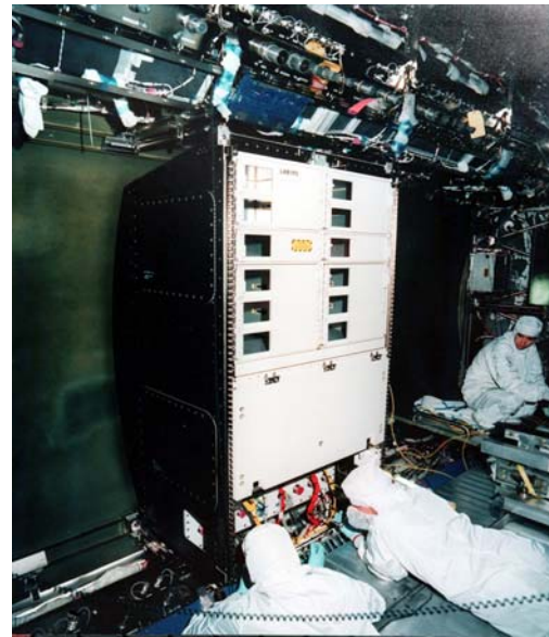
Figure 3. Destiny's first (EPS) system rack was installed in March 1998. The rack is pivoted at the lower standoff, and latched to the upper standoff. Boeing technicians connect power, data, and cooling lines and ducts between the lower standoff and the rack's ISPR standard panel.
