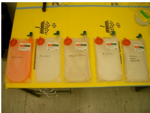
Figure 3 FO flux test run in progress evaluating four different liquid food products as the osmotic agent and seawater as source water in the LWC-WRS application.
