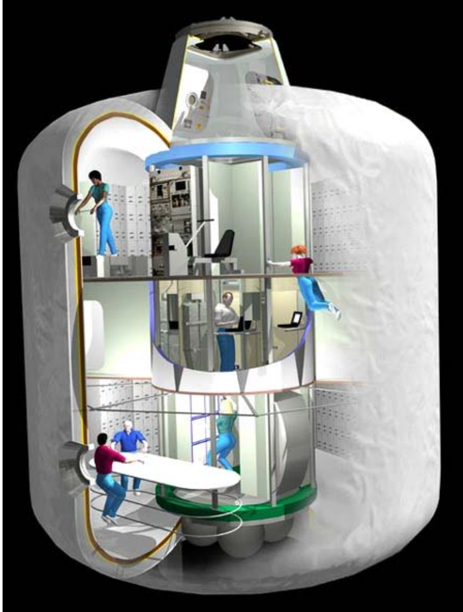
Figure 4: NASA's Proposed TransHab Module. Above is a conceptual drawing of the compartmentalized inflatable TransHab module that would have replaced current crew quarters onboard the International Space Station. 3
