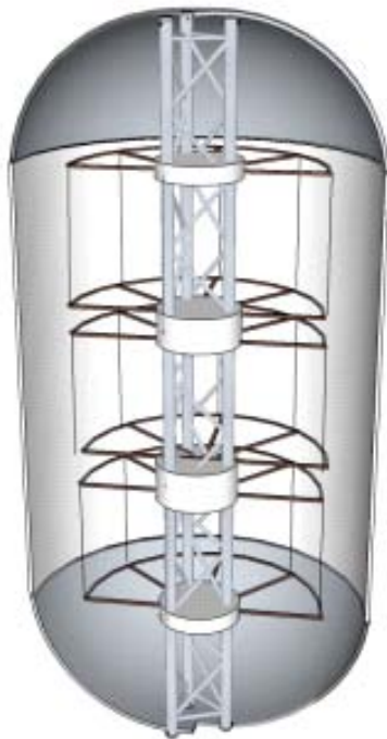
Figure 6: Farm module with pole structure extended. The above image shows the extended pole structure, which will deploy using a spring-loaded system. Once the structure has deployed, experiment boxes will fit between the poles and lock into place.
