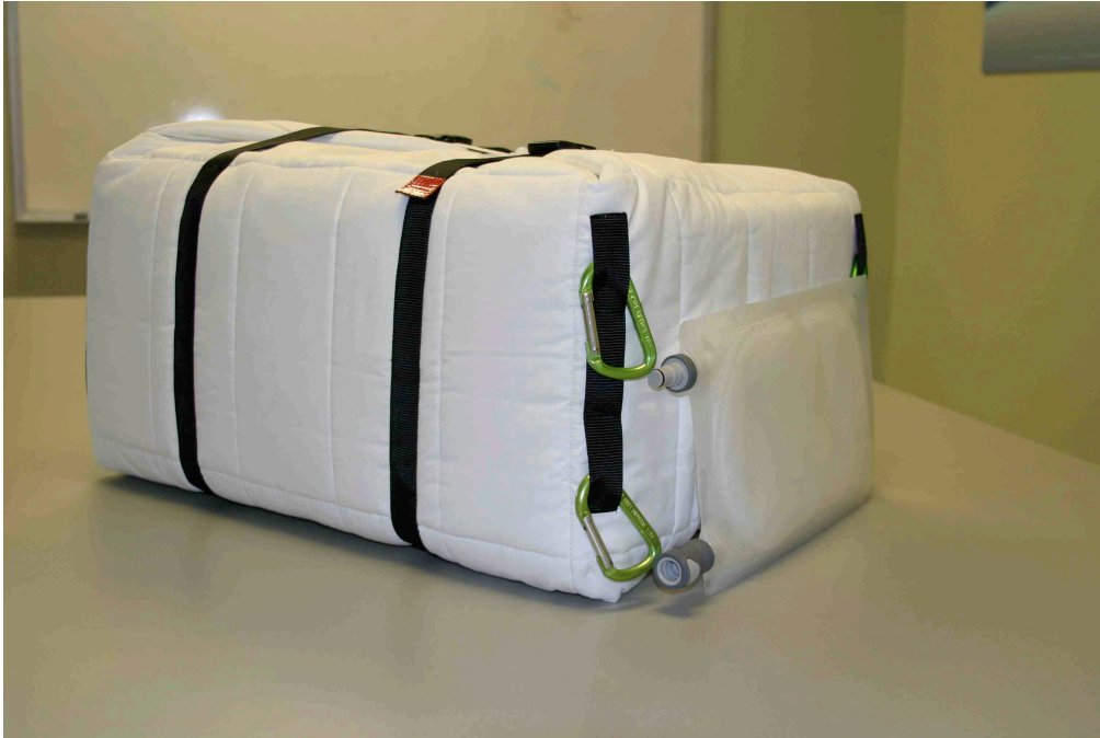
Figure 1: Folded FO-CTB water wall architecture element demonstrator.
