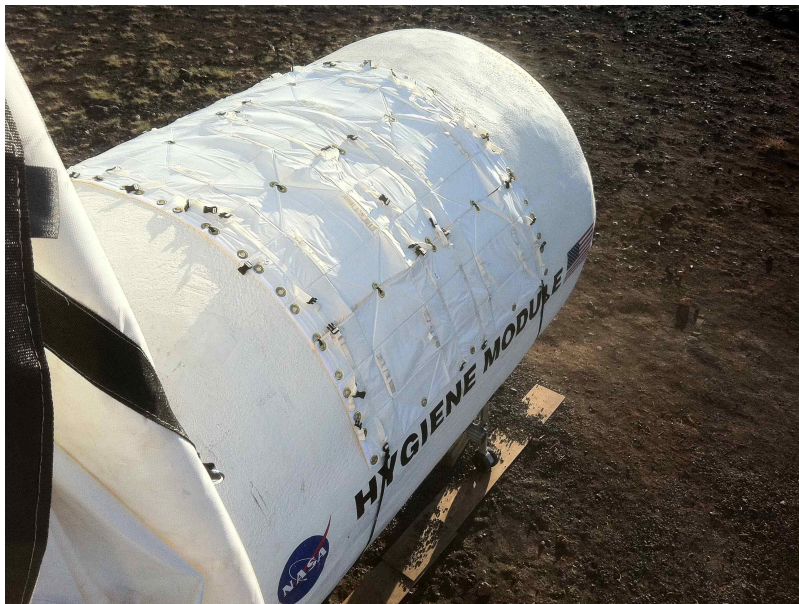
Figure 8: Exterior radiation sheading CTB mounting demonstration
