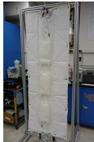
Figure 3: Unfolded FO-CTB water wall showing FO bags and plumbing.
