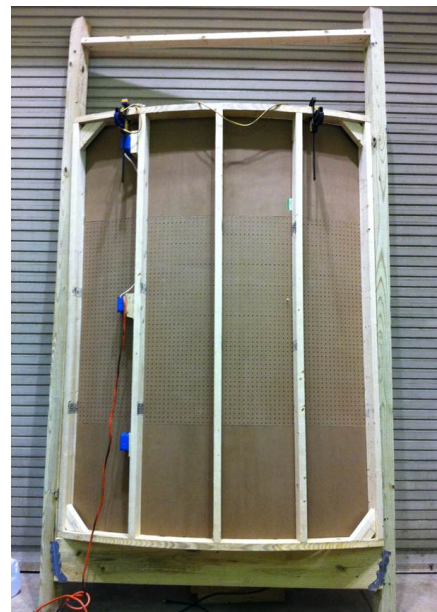
Figure 5. Wall section inserted into main structure element
