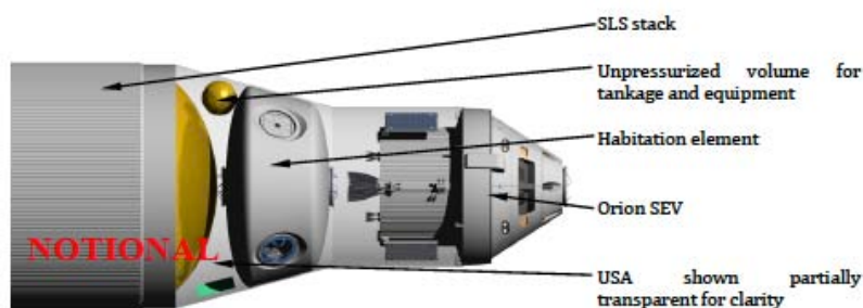
FIGURE 30. Evolvable Mars Campaign: frustoconical monolithic “large habitat” with four radial ports inside the dynamic envelope of an SLS payload shroud that is sized to match the diameter of an Orion (Courtesy of Matthew Simon, NASA LaRC).
