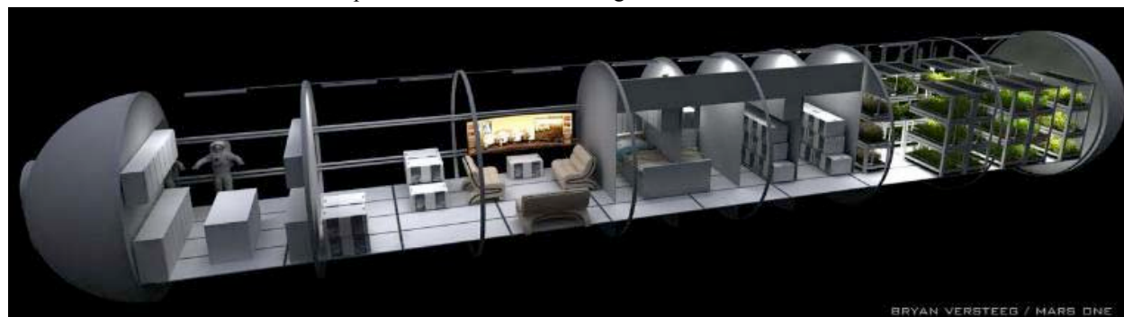
FIGURE 29. Longitudinal, cutaway view of the MarsOne 500 m 3 habitation and plant growth inflatable module. (Credit: Bryan Versteed, MarsOne).
