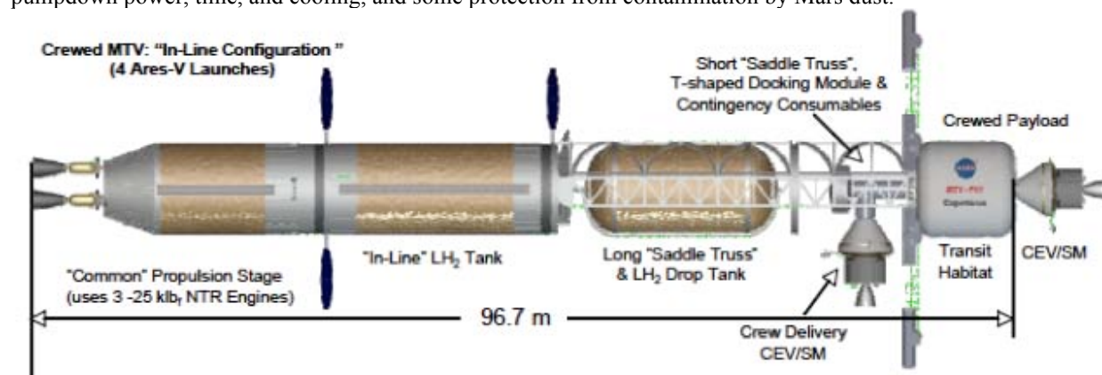
FIGURE 27b. NASA MDRA 5.0, an interplanetary vehicle that flies the crew round-trip from Earth to Mars. The habitat is a TransHab. The side-docking Orion CEV behind the habitat appears to derive from the IPV in Cohen, 1997a, p. 24.
