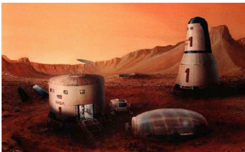
FIGURE 3. Robert Zubrin’s Mars Direct minimalist concept showing the basic elements of the lander/ascent vehicle, the crew habitat, inflatable greenhouse, and rover (Courtesy of the Mars Society).
