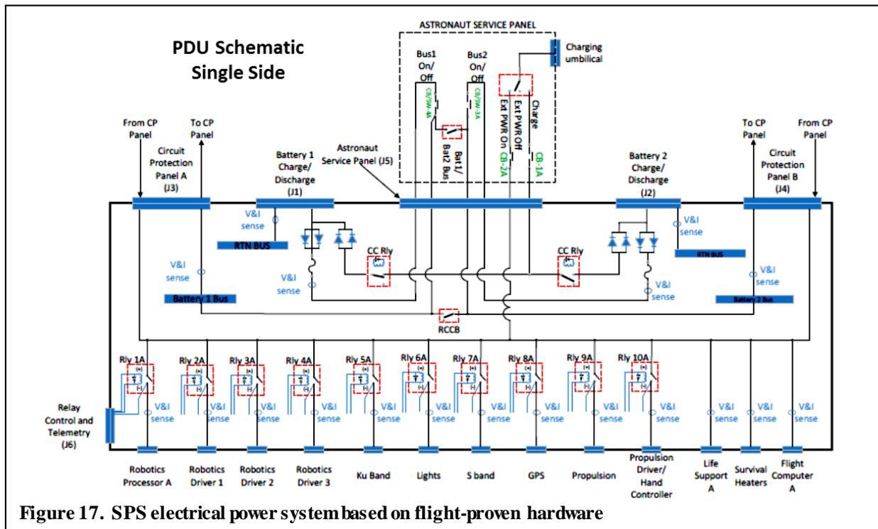
**Figure 17. SPS electrical power system based on flight-proven hardware**
