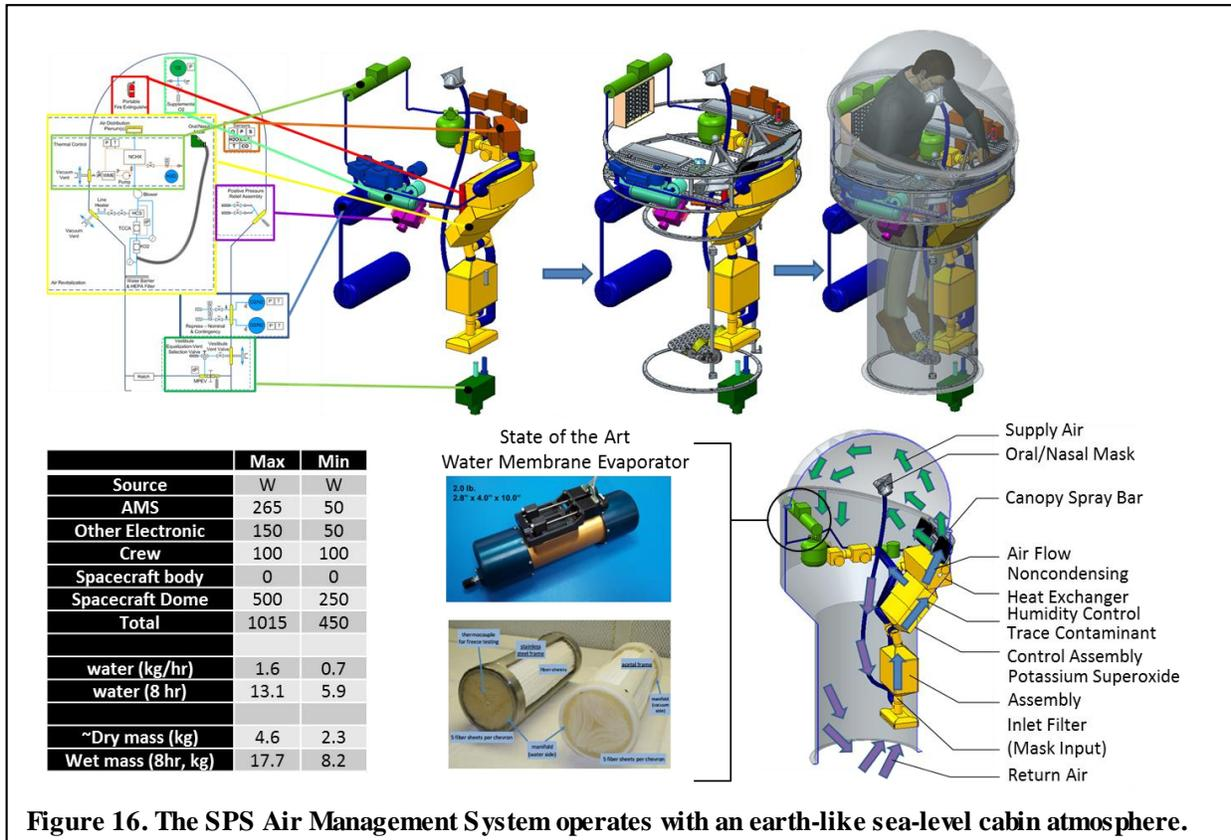
Figure 16. The SPS Air Management System operates with an earth-like sea-level cabin atmosphere.
