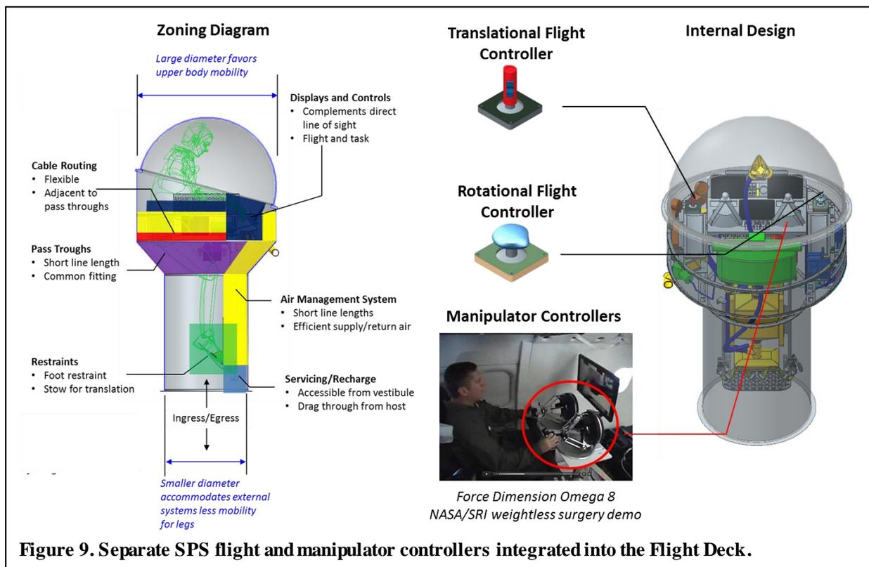
**Figure 9. Separate SPS flight and manipulator controllers integrated into the Flight Deck.**
