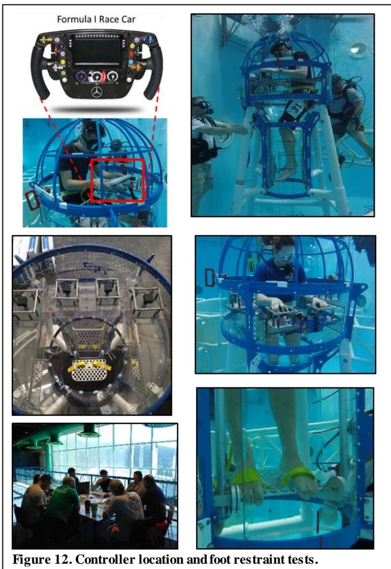
**Figure 12. Controller location and foot restraint tests.**
