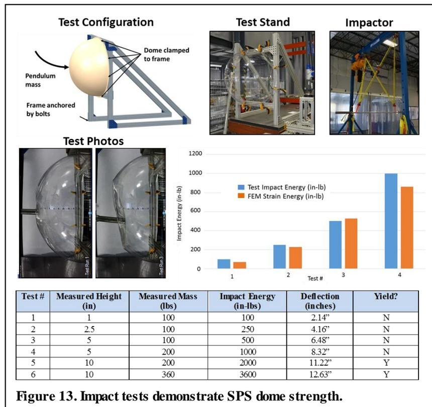
**Figure 13. Impact tests demonstrate SPS dome strength.**
