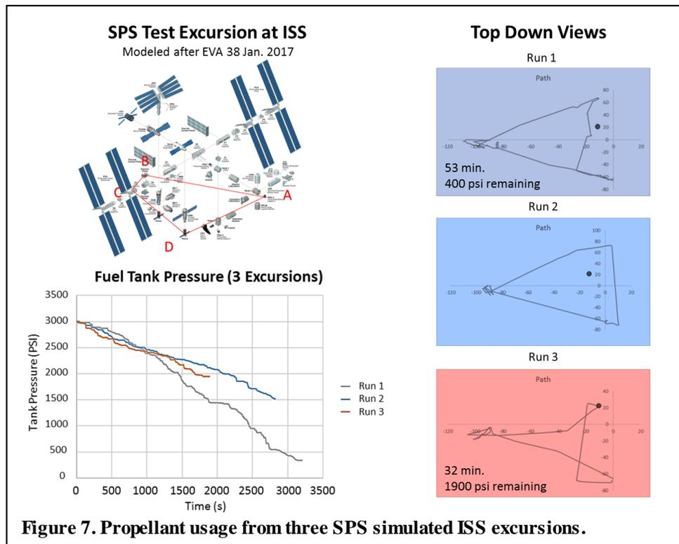
**Figure 7. Propellant usage from three SPS simulated ISS excursions.**
