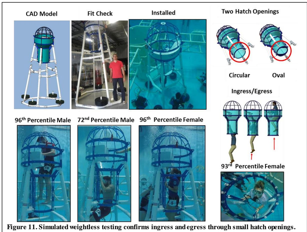
**Figure 11. Simulated weightless testing confirms ingress and egress through small hatch openings.**
