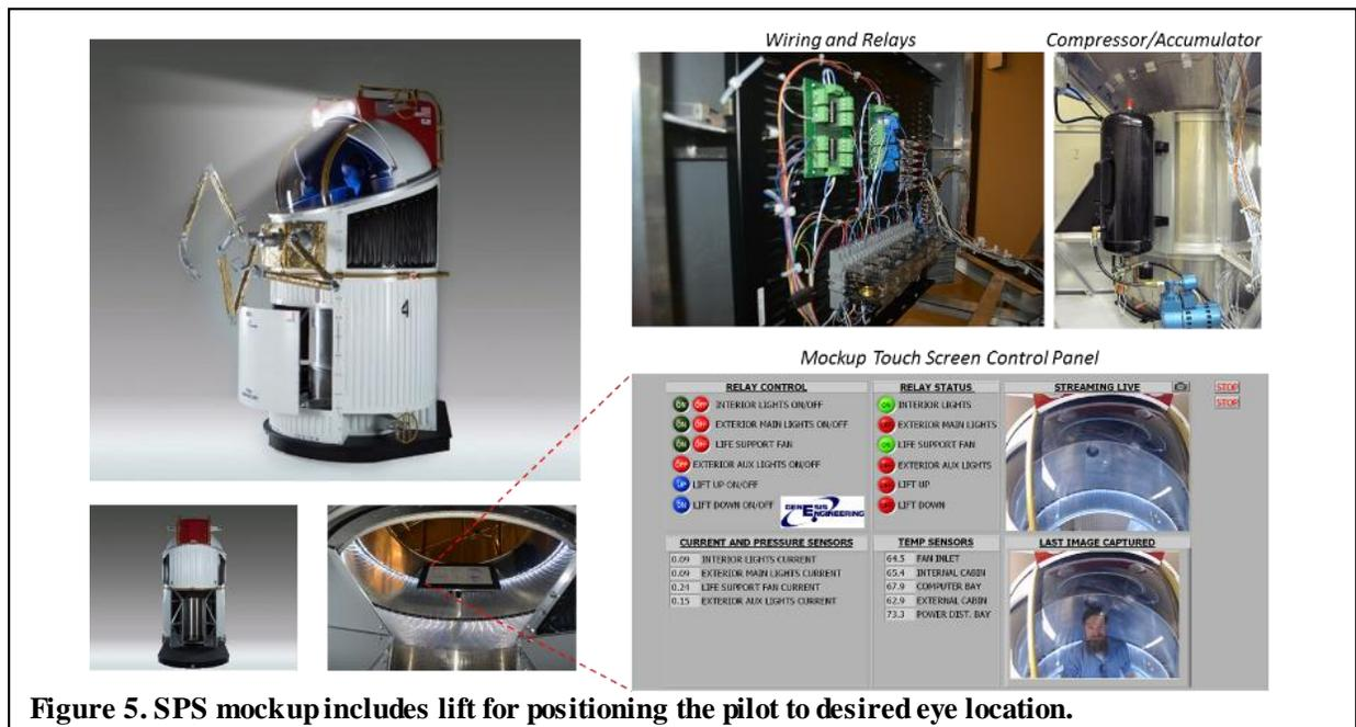
Figure 5. SPS mockup includes lift for positioning the pilot to desired eye location.
