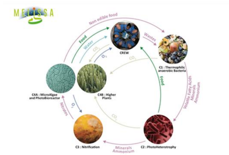
The closed-loop regenerative approach of the MELiSSA project (courtesy of the MELiSSA Foundation)
